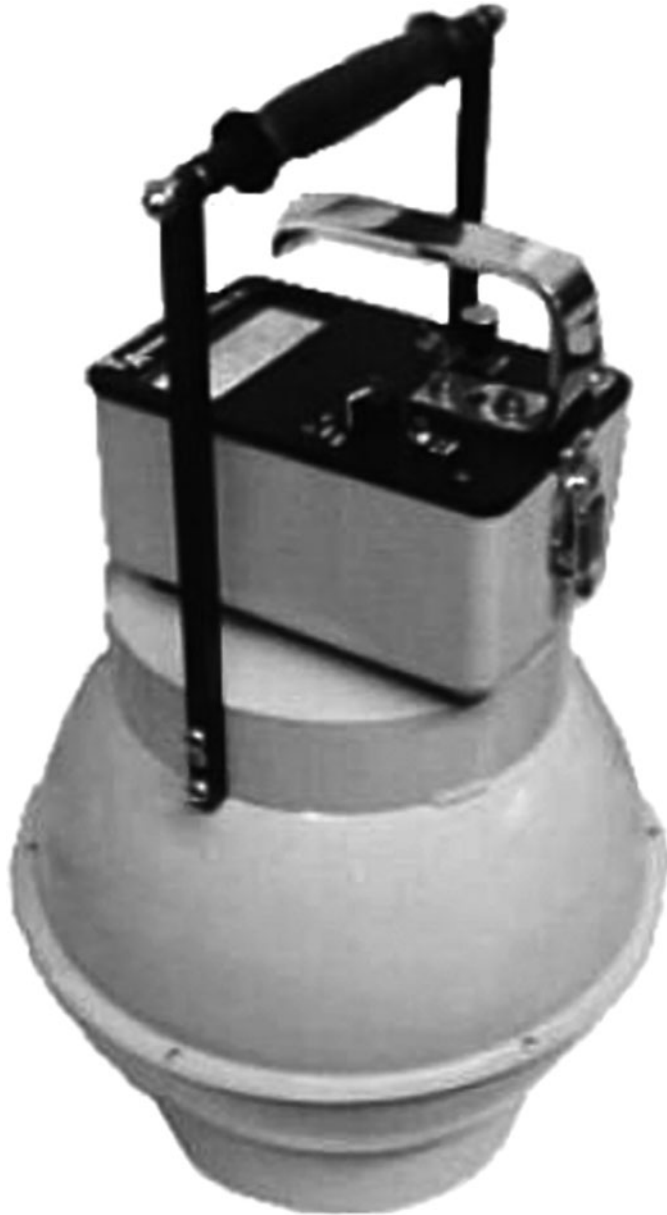
Figure 9-35. Spherical neutron dose-equivalent meter. The sphere is made of polyethelene, 10 inches diameter. The thermalized neutrons are measured with a ^3\text{He} filled detector. (Courtesy Technical Associates, Canoga Park, CA.)
