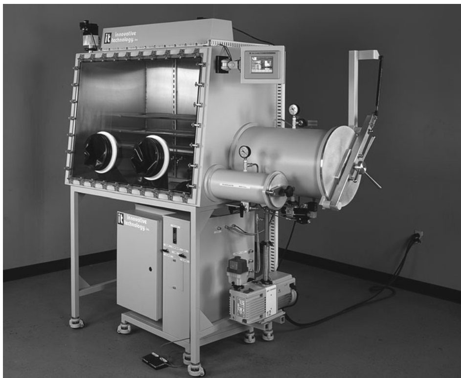
Figure 11-2. Glove box for operations with low-intensity radioactive materials that might accidentally become dispersed into the environment if not handled in an enclosed volume. In use, long rubber gloves fit over the port flanges; material transferred into or out of the glove box through the air lock at the right of the glove box. (Courtesy of Innovative Technology, Inc.)
