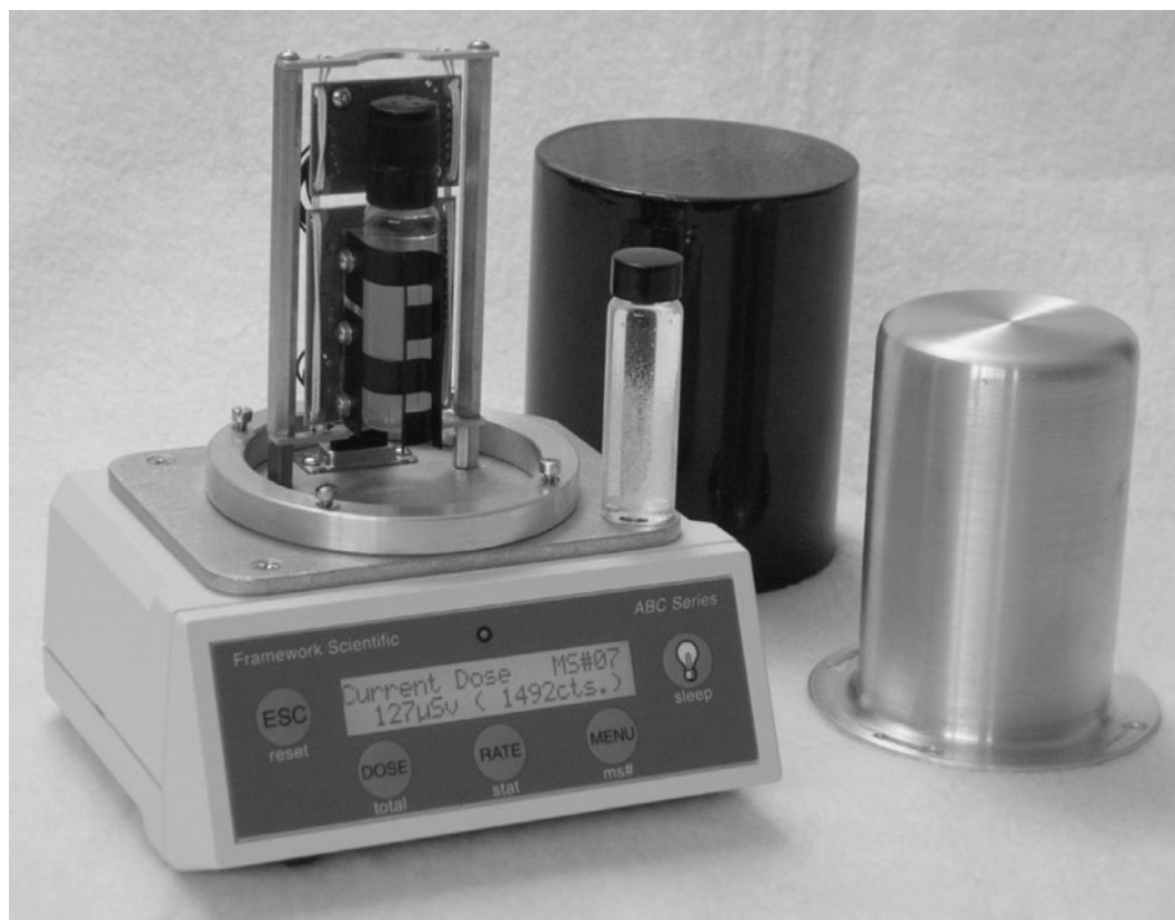
Figure 9-36. Photograph of a superheated emulsion vial and acoustical bubble counter. The lead cylinder in the background is used to extend the response to over 1 GeV. (Courtesy of FrameSci.com.)
