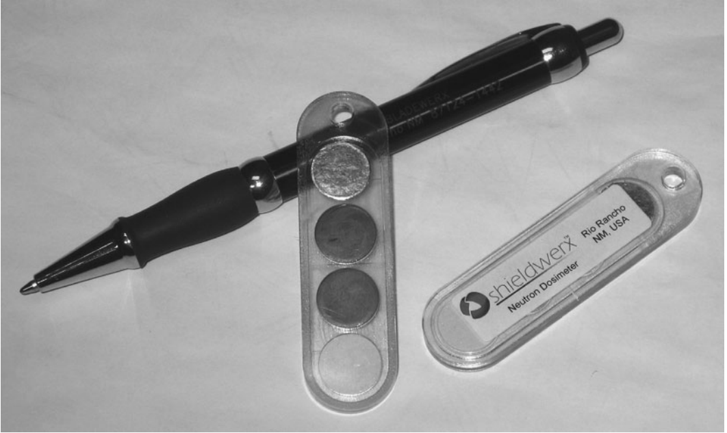
Figure 9-29. Pocket criticality dosimeter for measuring neutron exposure. Inside the dosimeter are four different foils whose induced radioactivity, following exposure to neutrons, depends on the neutron energy and fluence. (Courtesy of Bladewerx, LLC, Rio Rancho, NM.)
