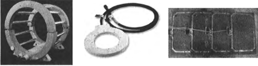
FIGURE 4.24. Three RF coils used for magnetic resonance imaging. (Left) a birdcage coil used for brain imaging, (center) a surface coil used for imaging close to the surface of the body, (right) a phased array used for spine imaging.
