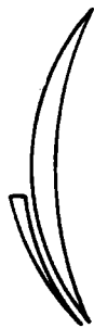
FIGURE 8-24. An Executive-style bifocal considered as a single-vision distance lens with a reading segment.
