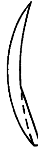
FIGURE 8-23. An Ultex-style bifocal, showing the imaginary surface dividing the segment and the major lens in the near portion of the lens.
