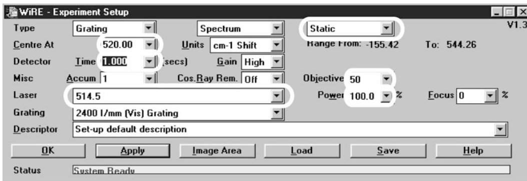
Fig. 9. WIRE/GRAMS software settings for measuring the Silicon reference spectrum.
