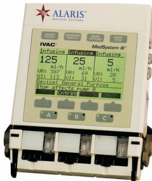
Figure 3-25 Infusion pumps apply pressure to deliver a set volume of liquid every minute.
