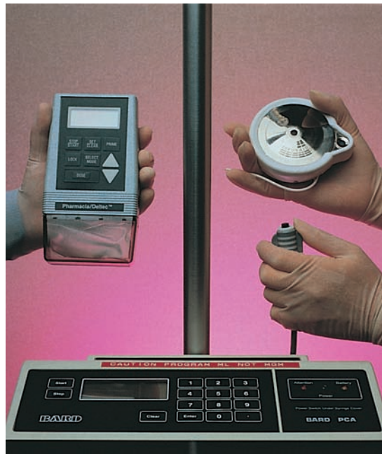
Figure 3-27 A patient-controlled analgesia (PCA) pump gives the patient limited control over the amount of medication administered.
