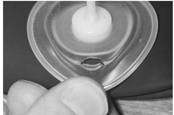
Figure 4.5 Silicone rubber diaphragm of the relief valve on the top of the bellows housing of the Dräger Large Animal Control Center anesthesia machine. During inspiration when the valve was shut by gas (oxygen) under pressure, the rip allowed fresh gas devoid of anesthetic to enter the bellows and dilute anesthetic gas in the bellows thus decreasing the concentration of anesthetic being delivered to the patient.
