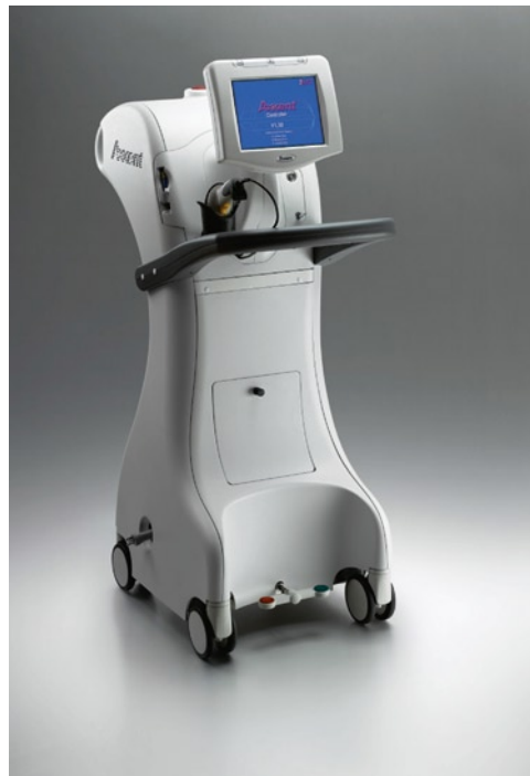
Fig. 5.4 Controller unit for the Axxent electronic brachytherapy system, which includes a touch-screen monitor, USB port, pull-back arm, bar-code scanner, X-ray source cooling pump, well chamber and electrometer. The USB port is for communicating dwell files and storing log files. The pull-back arm is an adjustable arm with a high-voltage port for the source connection.
