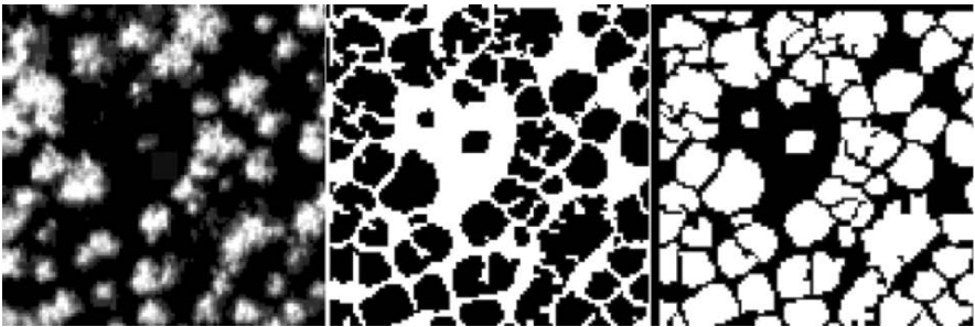
Figure 2-2. Left: Multi-detector Electro-optical Imaging Sensor (MEIS) 31 cm pixel image of part of the Hudson Plantation at the Petawawa National Forestry Institute, Ontario, Canada. Middle: Initial results of applying a valley-following program to identify trees. Right: Final results after applying a rule-based crown delineation program, which modifies the initial crown delineation results, for example by separating segments that have deep embayments. (Reprinted from Canadian Journal of Remote Sensing Vol. 21, F. A. Gougeon, 1995. A crown-following approach to automatic delineation of individual tree crowns in high-spatial-resolution aerial images, pp. 274-284. Used with the permission of the Canadian Aeronautics and Space Institute.)
