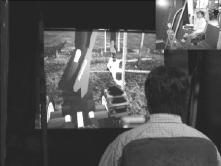
Figure 5-9. Harvest simulator used for training machine operators.
