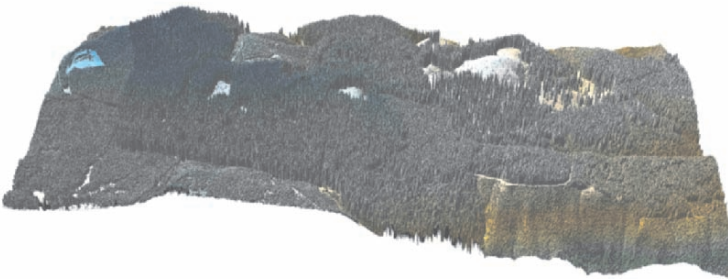
Figure 3-5. Shaded relief of the LIDAR-derived canopy surface model for Capitol Forest study area, Washington, USA. (See also color plate 3-5 on p. CP3)
