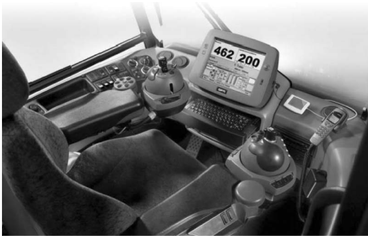
Figure 5-10. Inside the cab of a modern harvester with sensing, computing, and communications technologies (Courtesy of Ponsse Oy).
