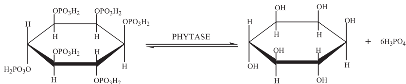
FIGURE III.29. Structure showing the enzymatic hydrolysis of phytic acid to inositol and phosphoric acid by phytase
