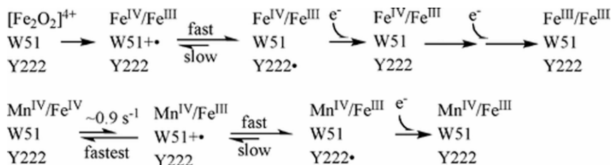
Figure 12. Proposed mechanism for electron relay to the binuclear Mn–Fe cofactor of the R2 subunit of Chlamydia trachomatis during O 2 activation by Fe(II)–Fe(II) form (top) of R2 and the Mn(II)–Fe(II) (bottom) form of R2. Reprinted with permission from [69]. Copyright © 2008, American Chemical Society.
