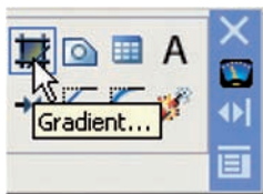
Fig. 8.7 The Gradient Hatch tool icon from the 2D Draw control panel
