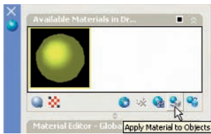
Fig. 16.20 The Apply Material to Objects button in the MATERIALS palette
