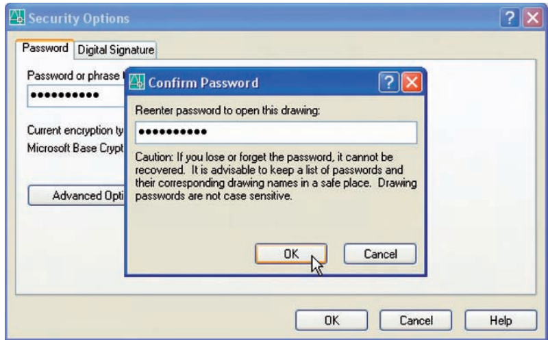
Fig. 21.2 Entering and confirming a password in the Security Options dialog
