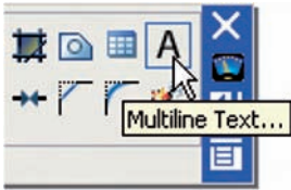
Fig. 6.35 The Multiline Text tool icon from the 2D Draw control panel
