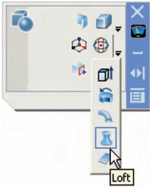
Fig. 13.39 The Loft tool icon in the 3D Make control panel
