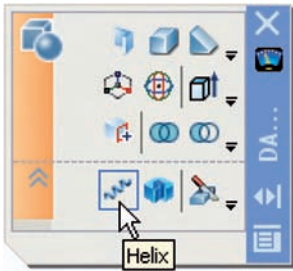
Fig. 15.38 The Helix tool icon in the extension of the 3D Make control panel
