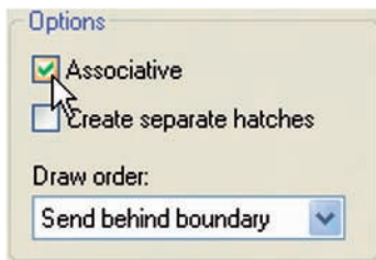
Fig. 8.6 Associative hatching set ON in the Hatch and Gradient dialog
