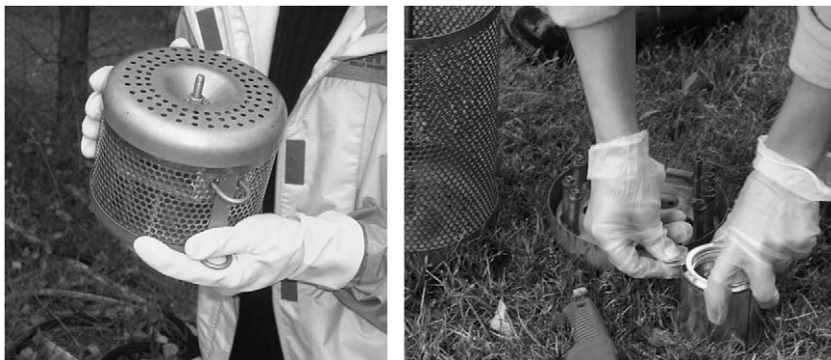
Fig. 14.5. A commercially available stainless steel deployment canister that holds a maximum of two SPMD racks and an airtight tin can for storage of membranes.
