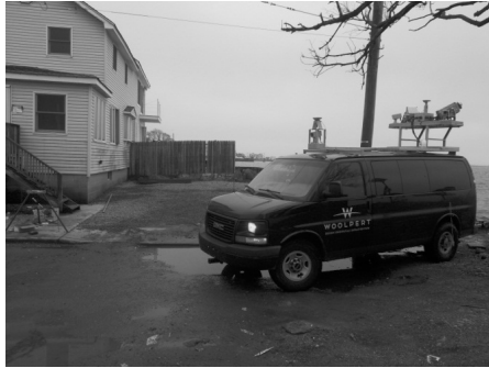
Figure 2. The Mobile LiDAR Data Collection Van
