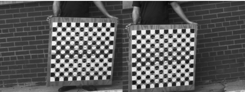
Figure 3: Automatically detected and matched calibration board corners
