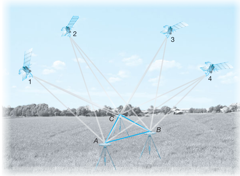
Figure 14.8 GNSS observation session using three receivers. In the case shown, AB and BC are considered nontrivial baselines. Thus, AC is a trivial baseline.
