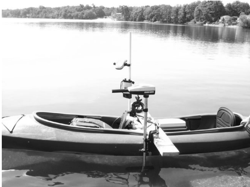
Figure 17.13 Depth sounder used in small lake hydrographic survey. (Sea Floor Systems, Inc.)
