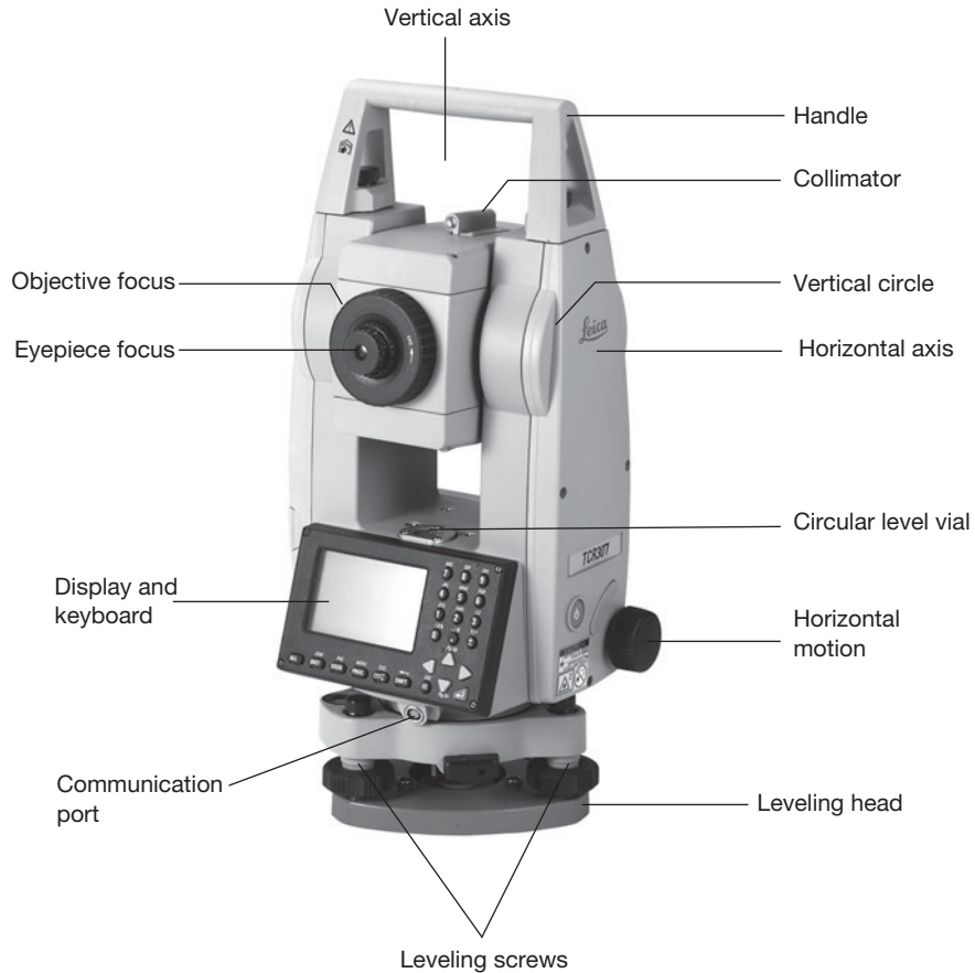
Figure 8.1 Parts of a total station instrument, with view of eyepiece end of telescope. (Courtesy Leica Geosystems AG.)
