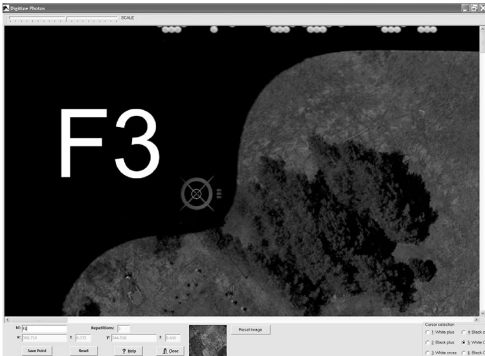
Figure 27.23 The observation of fiducial F3 in the WOLFPACK photogrammetric software.
