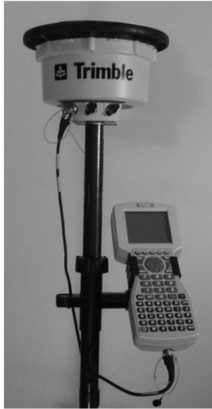
Figure 14.3 GPS antenna attached with cables to controller unit. (Courtesy of Trimble.)
