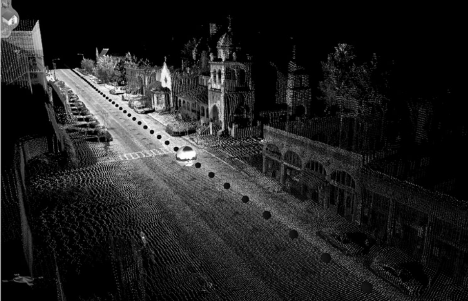
Figure 17.11 Point cloud from the IP-S2 3D mobile mapping system. (Courtesy Topcon Positioning Systems.)
