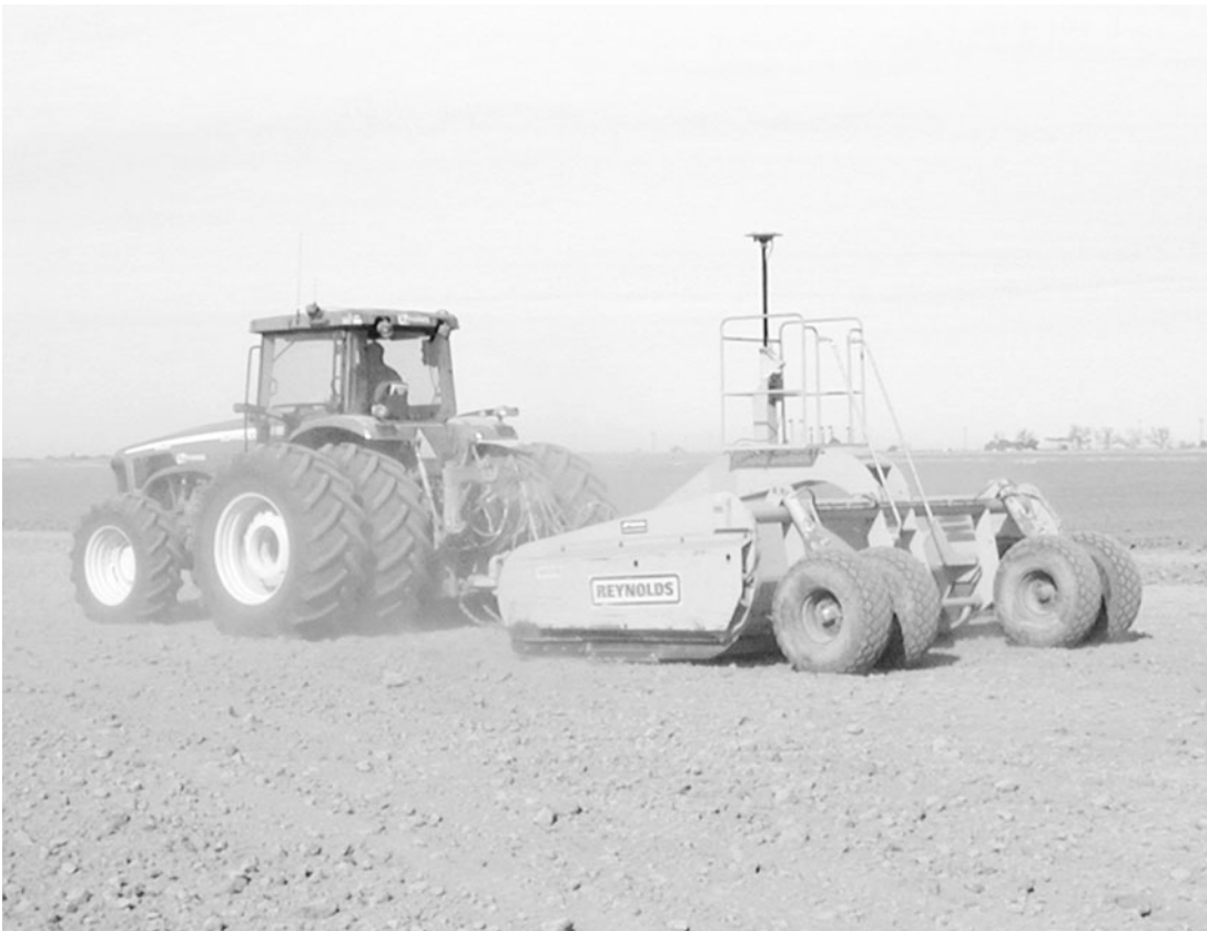
Figure 15.8 A large tractor pulling a land leveler. (Courtesy Topcon Positioning Systems, Inc.).
