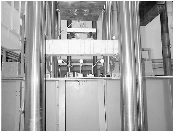
Figure 1 Test setup of a short beam (span = 1m)
