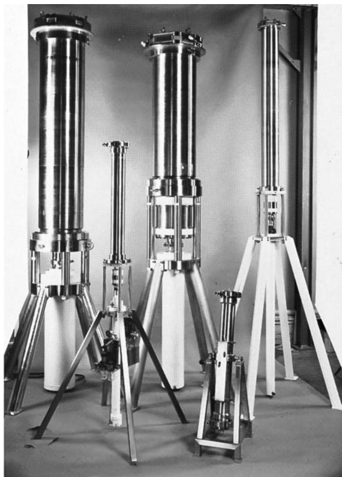
Figure 19.6. Stainless steel columns for liquid chromatography (37) . Two are 450 mm dia., one 150 mm dia. and two 110 mm dia. Pressure rating 70 bar. The devices below each column permit axial bed compression by piston
