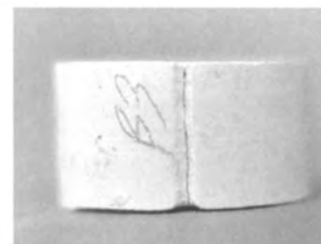
Fig. 5. The Brazilian Crushing Strength of chalk.
