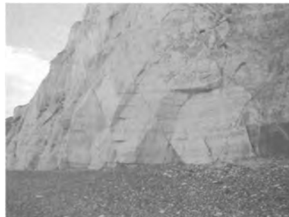
St Martin Plage, Holywell Chalk, steeply inclined conjugate joints. Note dihedral angle and frequency of joints compared to New Pit Chalk above
