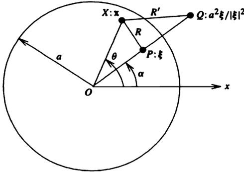
Fig. 5.4 Image points in a circle or sphere.
