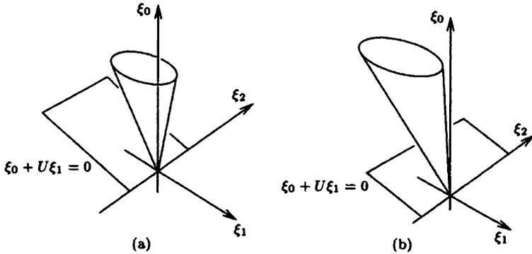
**Fig. 2.18** Normal cones for (2.57) when (a)  $U < a_0$  and (b)  $U > a_0$ , with  $\xi_0 = t$ ,  $\xi_1 = x$  and  $\xi_2 = y$ , so that  $(\xi_0 + U\xi_1)((\xi_0 + U\xi_1)^2 - a_0^2(\xi_1^2 + \xi_2^2)) = 0$ .
