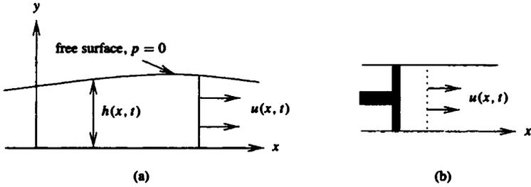
Fig. 2.1 (a) Open channel shallow water flow; (b) one-dimensional unsteady gas flow driven by a piston.
