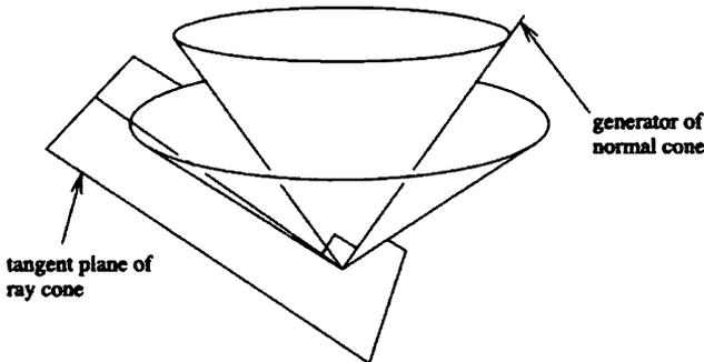
Fig. 2.17 Normal and ray cones.
