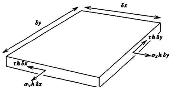
Fig. 2.4 Glass sheet stretching: force balance.
