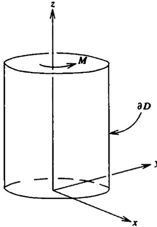
Fig. 5.1 Torsion of a bar.
