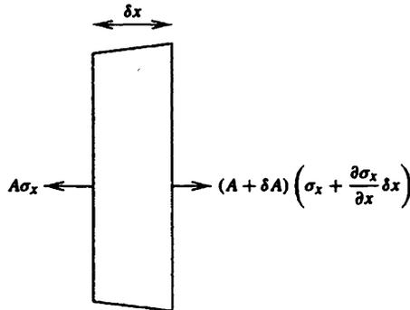
Fig. 2.3 Fibre-drawing: force balance.
