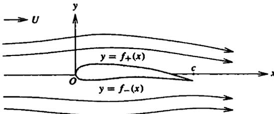
Fig. 5.2 Flow past an aerofoil.
