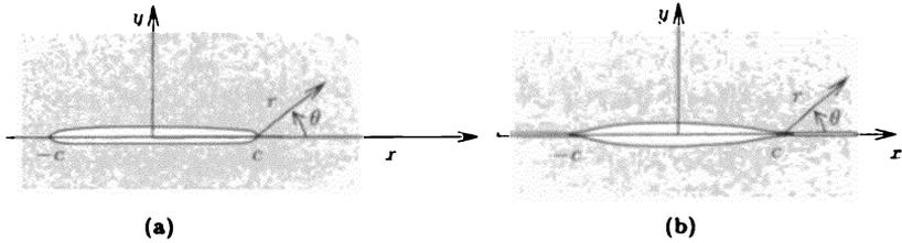
**Fig. 5.3** (a) Brittle fracture in pristine material; (b) partly opened pre-existing crack.
