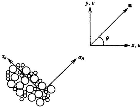
**Fig. 2.5** Flow of a granular medium;  $\sigma_n$  is the normal stress and  $\tau_\theta$  the shear stress on a surface with normal  $\mathbf{n}$ .
