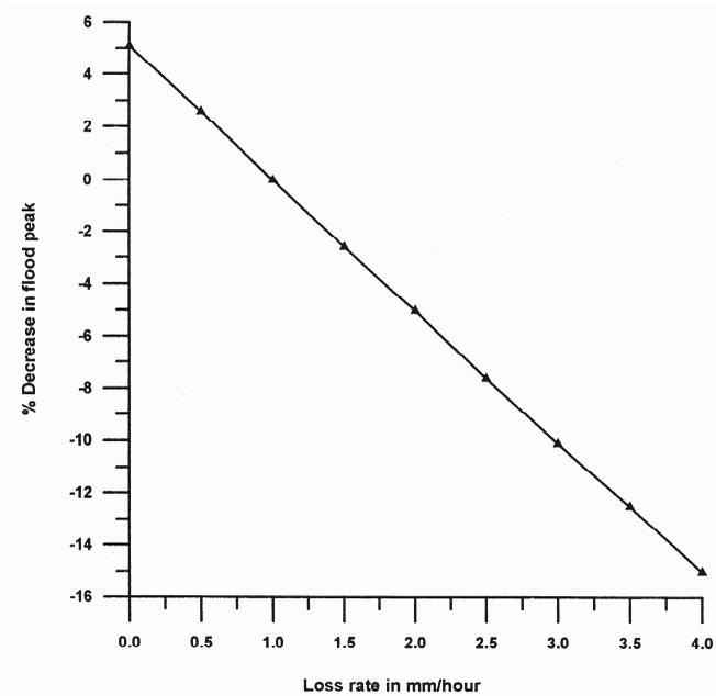
**Figure 10.17.** Variation of percentage decrease in flood peak with loss rate
