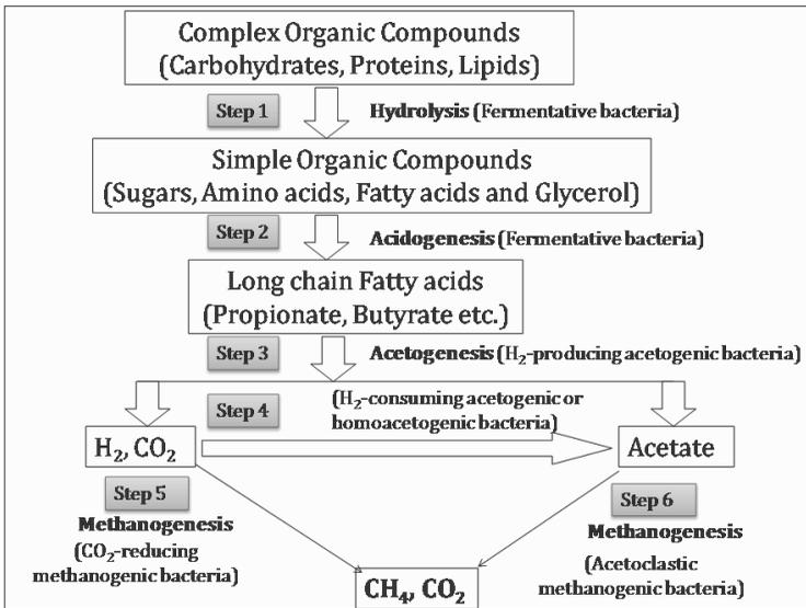
**Figure 24.9.** Metabolic steps and microbial groups involved in anaerobic digestion (modified from Novaes 1986)
