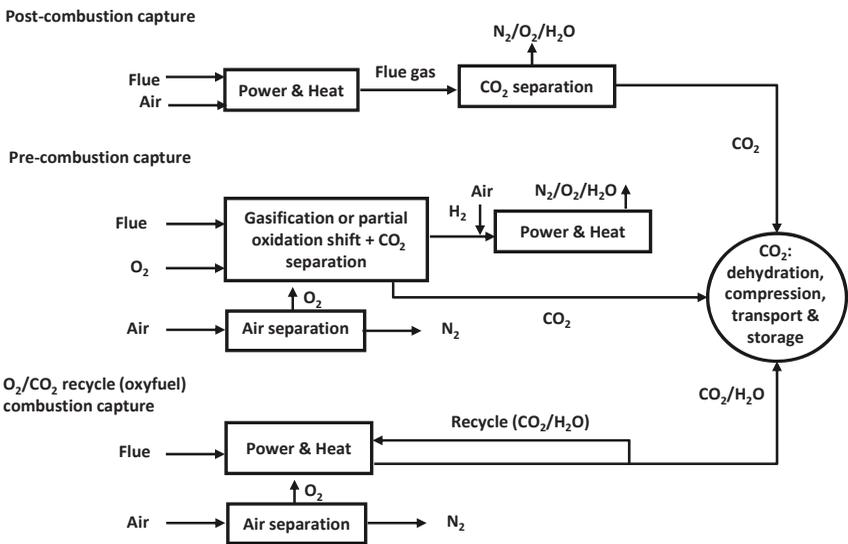
**Figure 20.1.** Overview of CO<sub>2</sub> capture from power plants (adapted from VGB 2004)
