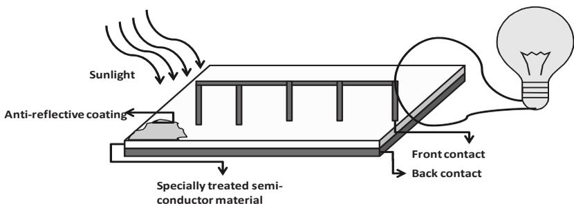
**Figure 24.7.** Schematic of a typical photovoltaic cell
