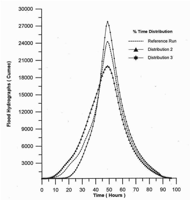
**Figure 10.16.** Design flood hydrographs for various percentage design storm distribution patterns
