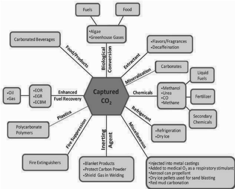
Figure 20.2. Schematic diagram of beneficial uses of CO<sub>2</sub> (Damiani et al. 2012)
