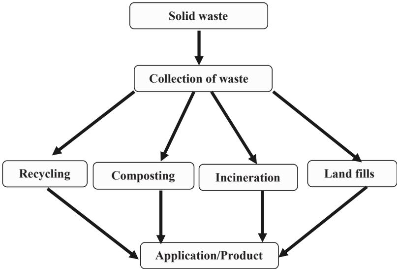
**Figure 23.2.** Flow diagram of an integrated solid waste management system
