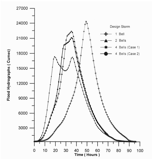
Figure 10.13. Design flood hydrographs for various storm patterns
