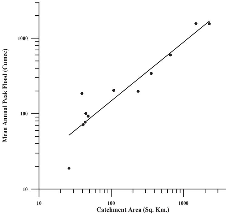
**Figure 10.5.** Variation of mean annual peak flood with catchment area for various gauging sites of Chambal Subzone 1(b)
