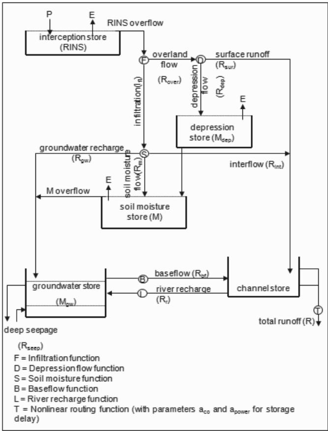
Figure 11.4. MODHYDROLOG model schematic
