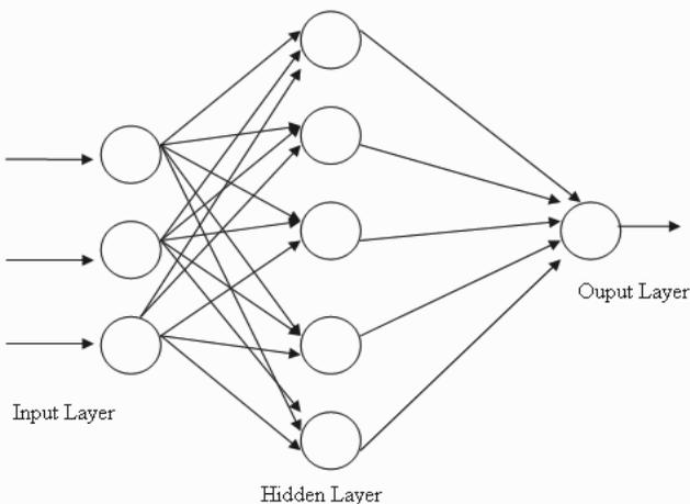
**Figure 9.1.** Three layer Feed-Forward Neural Network
