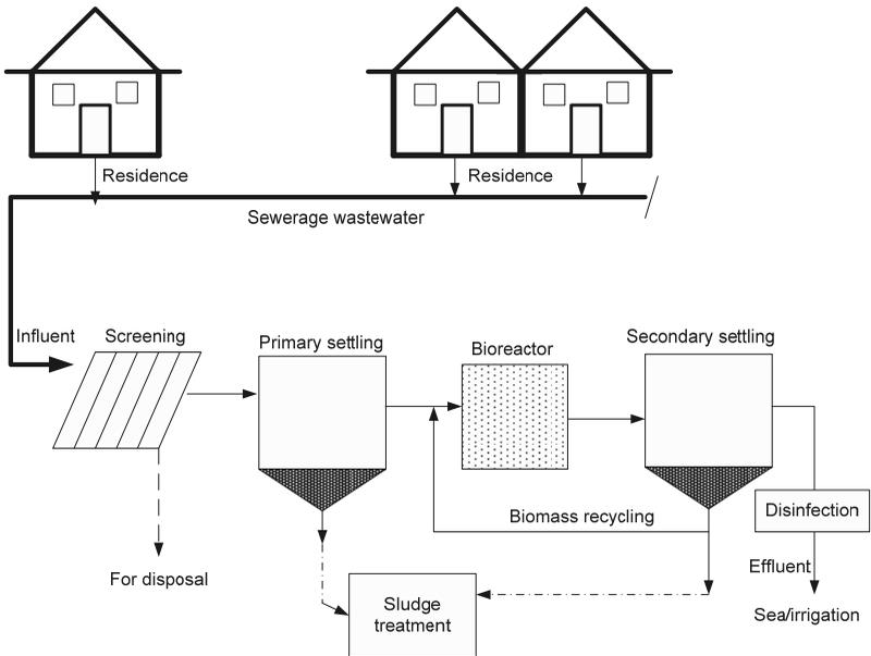
**Figure 21.1.** A typical wastewater treatment process
