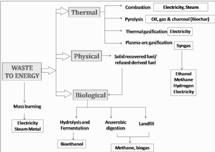
**Figure 24.8.** Different routes of transformation of waste to energy (modified from The Cleantech Report, 2007)
