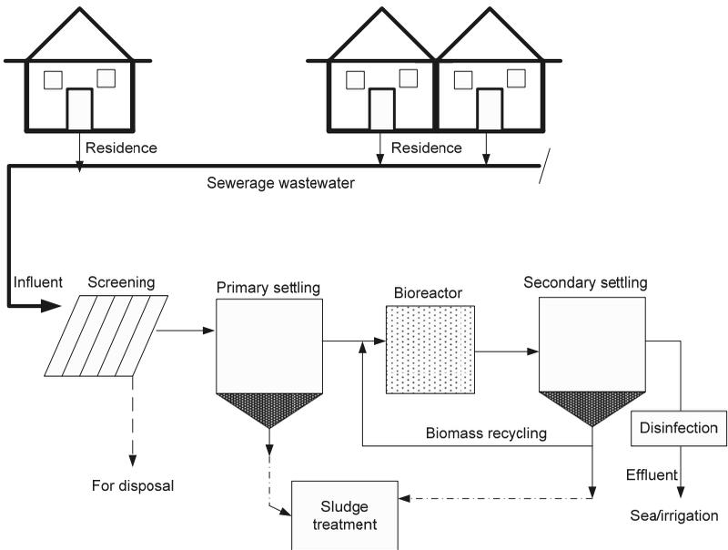
**Figure 21.1.** A typical wastewater treatment process
