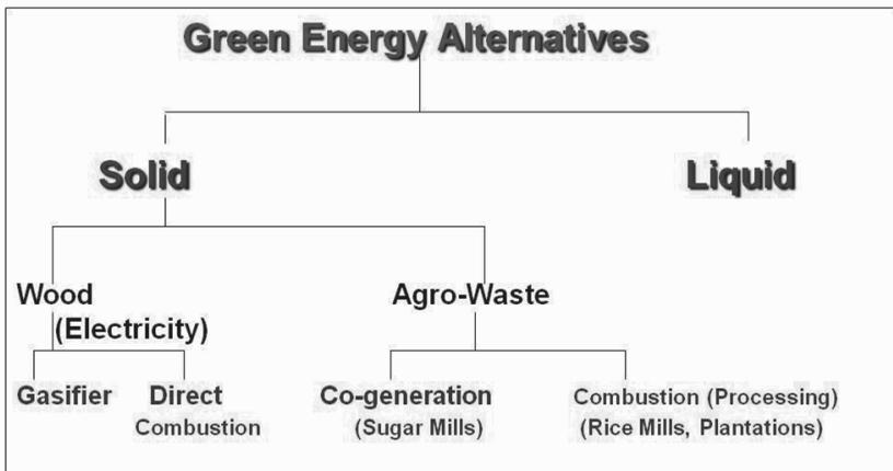
**Figure 24.5.** Schematic of biomass as green energy alternatives
