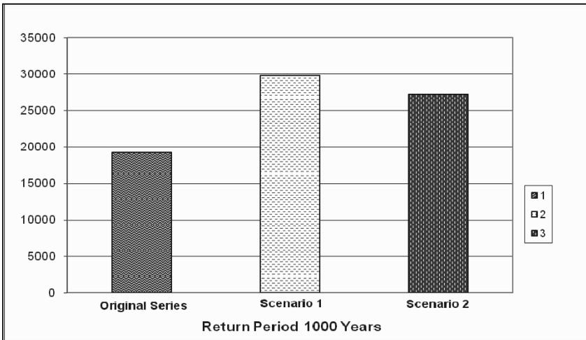
**Figure 10.8.** Comparison of floods for 1000 years return period floods for the original series and Scenario-1 and Scenario-2 under climate change
