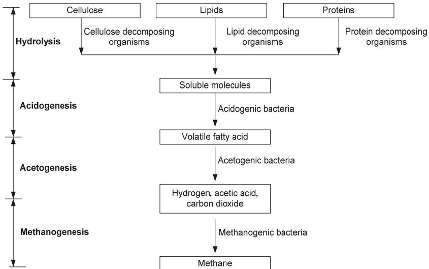
**Figure 21.2.** The degradation steps of the anaerobic digestion process
