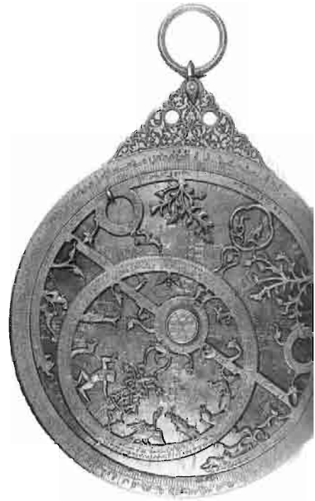
Astrolabe made in Cairo in 1236, engraved brass inlaid with silver and copper. The astrolabe was used by astronomers and astrologers throughout the Islamic world.
