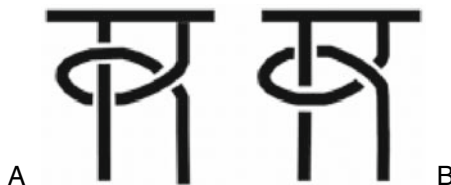
FIGURE 6.4. Half hitch configurations. (A) Under/over. (B) Over/under. (From Lo IKY. Essential Principle of Tying Secure Arthroscopic Knots. In: The Handbook of the 23rd Fall Course of The Arthroscopy Association of North America. Reprinted with permission.)
