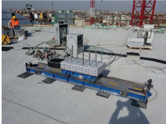
Figure 4 – Linear motor with slide and mass used as an actuator
