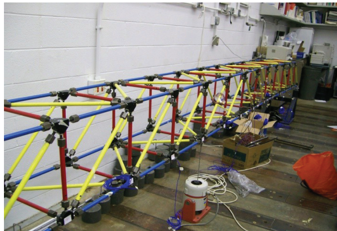
Fig. 7 Experimental truss with removable members in the Smart Structures Technology Laboratory at the University of Illinois
