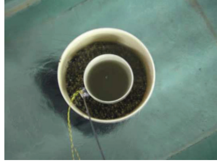
Fig. 4b Bridge model and the additional external cylinder with debris
