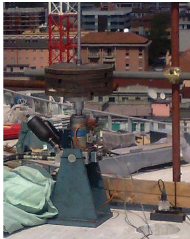
Figure 5 – hydraulic actuator and mass used
