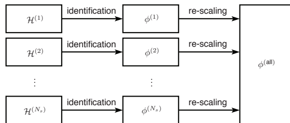
Fig. 1 Merging partial mode shape estimates \phi^{(j)} , j = 1, \dots, N_s into a global mode shape estimate \phi^{(all)} in the PoSER approach.
