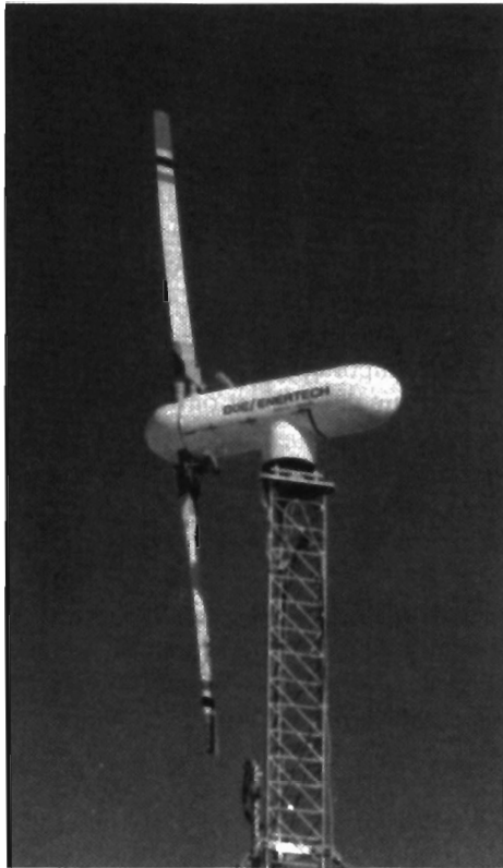
(a) Horizontal-axis wind turbine
