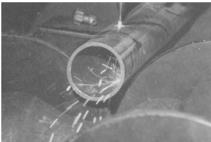
Figure 6.3 Flame cutting (Courtesy of Billington Structures Ltd)
