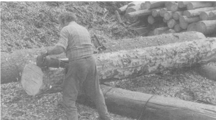
Figure 8.2 De-barking by hand prior to conversion
