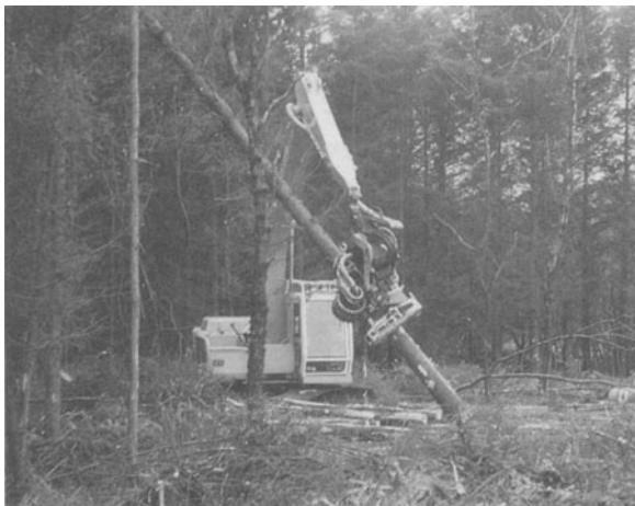
Figure 8.1 Mechanical harvester felling, de-limbing and cutting to length in one operation (Photograph courtesy of Fountain Forestry Ltd)
