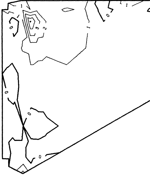
Fig. 5. Maximum principal stress contours Fault/snag condition - no dome; with gap
