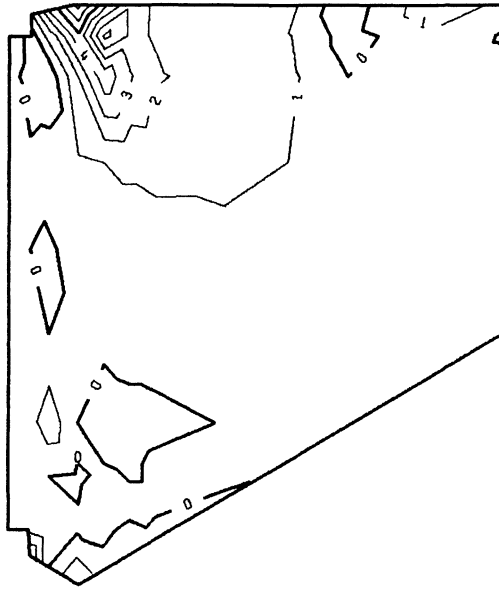
Fig. 7. Maximum principal stress contours Fault/snag condition - no dome; no gap
