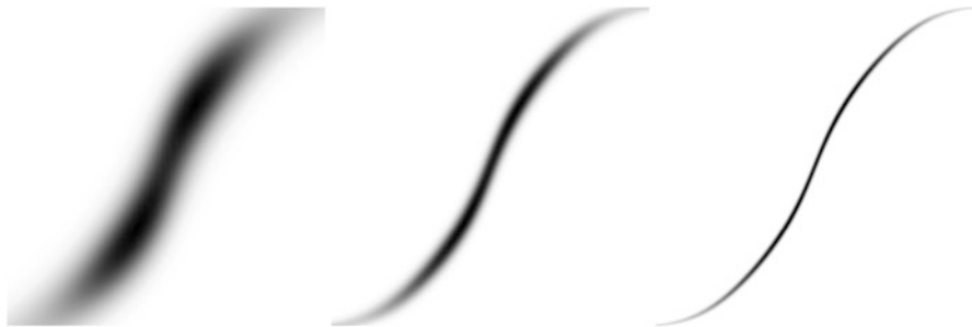
Fig. 6.2 The optimal \gamma in a 1D transport problem (the starting measure is a centered Gaussian; the arrival measure is composed of two bumps), via IPFP methods with decreasing values of \varepsilon . The image on the right gives a quite precise description of the optimal (monotone) map. Pictures kindly provided by L. Nenna
