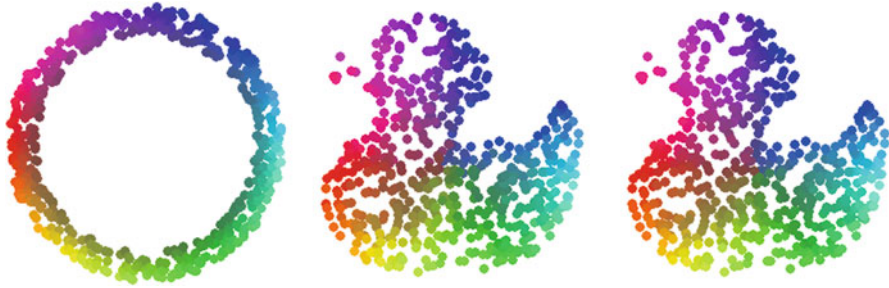
Fig. 2.5 Optimal transport between a finite number of points on an annulus and on a duck. Colors represent the assignment of points in the annulus to points on the duck. Middle, 1D-sliced assignment; right, optimal map for the quadratic cost. The two results are very similar (but one can find few points with different colors, which means a slightly different assignment). Picture taken from [256] with permission
