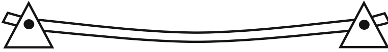
Figure 10.3: Physical problem leading to ODE (10.9): a beam bending under its own weight.
