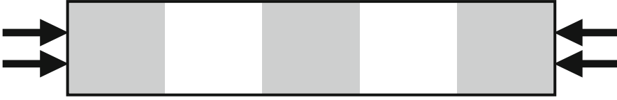
Figure 8.26: Schematic of buckles in a long rectangular plate under compression. The sign of the out-of-plane deformation alternates between shaded and unshaded regions, say upward in the shaded regions and downward in the unshaded regions.
