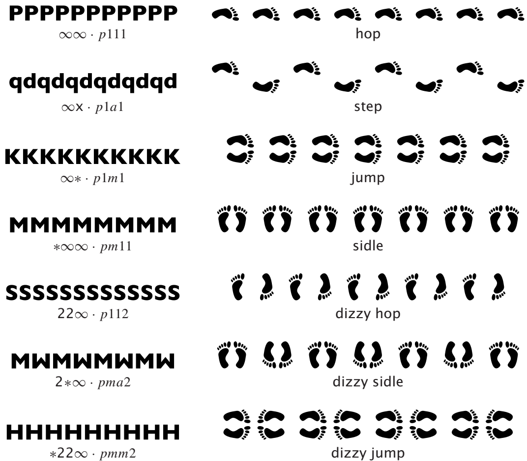
Figure 3.2: Examples of figures belonging to each of the seven frieze groups. The drawing on the left of each row is formed from letters, and is labeled both with its orbifold signature and the older crystallographic notation. The design on the right is formed from footprints and labeled with names suggested by Conway.
