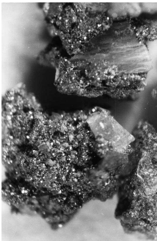
Fig. 4. Argillo-calcareous rock fragment containing huge amounts of pyrite particles.
