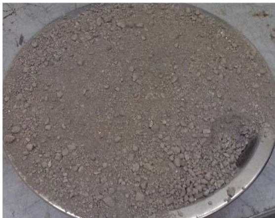
Figure 6.10 Slag as an aggregate, fraction 0–4 mm
