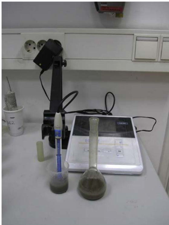
Figure 6.18 Measuring of the pH value of concrete eluate
