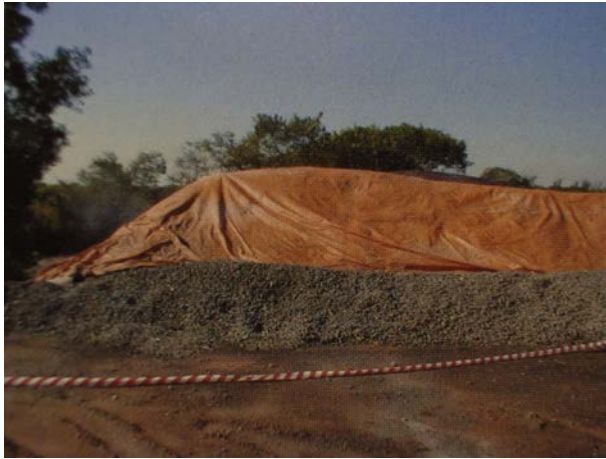
Figure 2.6 Accelerated slag ageing by steam exposure under a tarpaulin [25]
