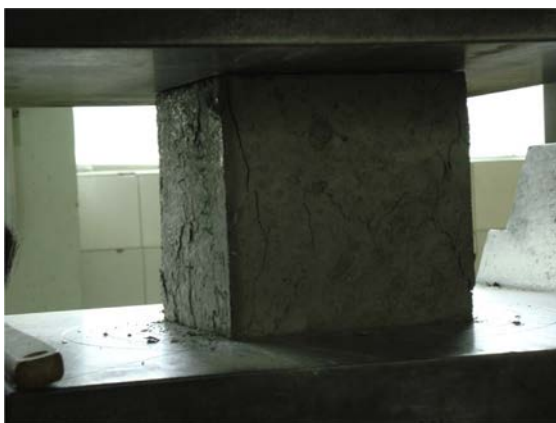
Figure 6.16 Compressive strength testing on concrete cubes with 15-cm edge lengths
