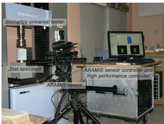
Figure 6.52 Test setup for 3D DIC measurement [33]
