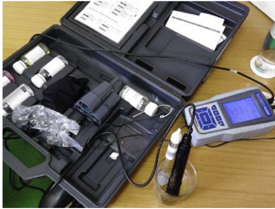
Figure 6.62 Leachate pH and DO measurement [65]
