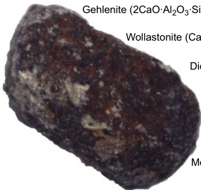
Figure 2.1 Minerals of air-cooled blast furnace slag [3]
