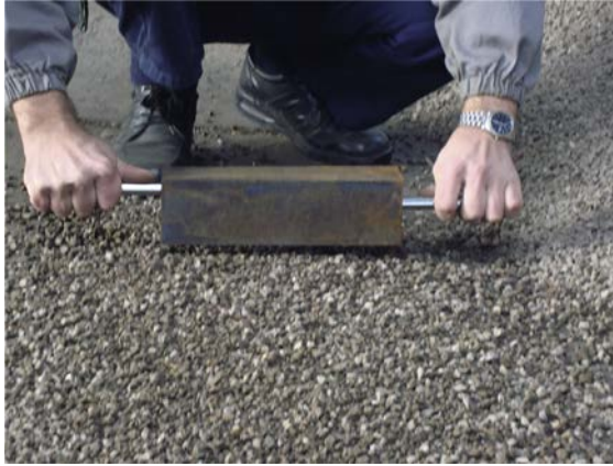
Figure 6.7 Using a magnet to select aggregate particles containing metals by hand
