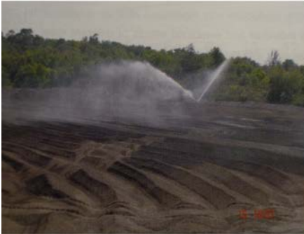
Figure 2.5 Accelerated hydration of instable components in slag; (a) slag splashing; (b) slag mixing [25]
