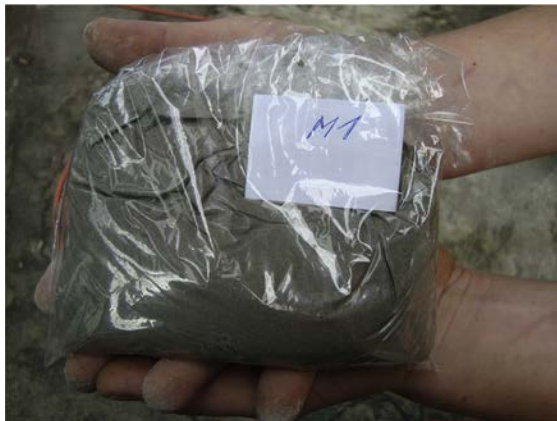
Figure 6.13 Sample of fresh concrete mixture for testing the pH value of concrete eluate
