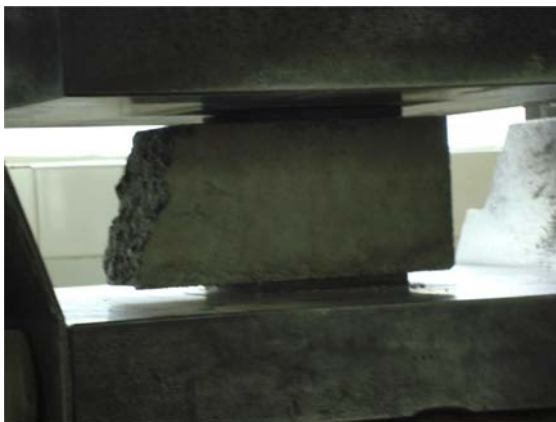
Figure 6.15 Compressive strength testing on prism halves
