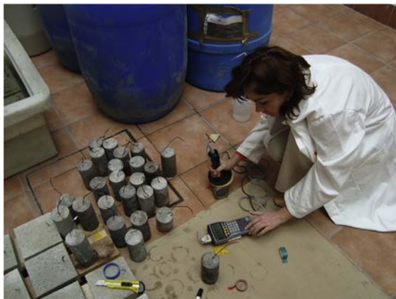
Figure 6.27 Measuring of corrosion parameters
