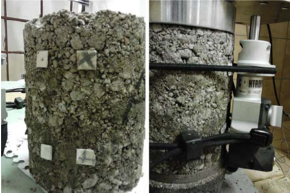
Figure 6.50 Sample with a mounted LVDT, demonstrating the difficulty of its positioning, and thus the questionable validity of the obtained results [33]
