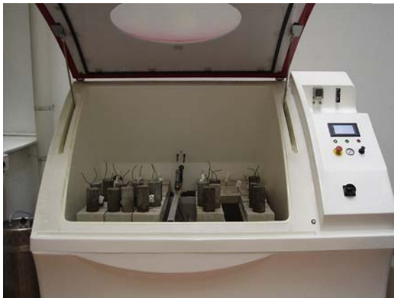
Figure 6.26 Samples exposed to a simulated marine environment in a salt chamber
