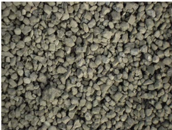
Figure 6.9 Slag as an aggregate, mix of fractions 4-8 and 8-16 mm
