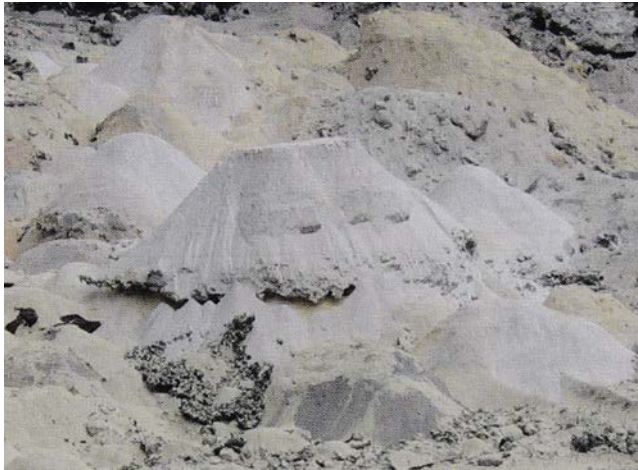
Figure 2.8 Decomposition of dicalcium silicate [28]
