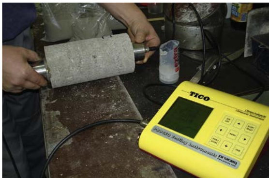
Figure 6.51 Ultrasonic pulse measurement of cement-stabilised steel slag mixtures [35]
