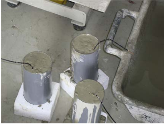
Figure 6.25 “Lollipops” with embedded reinforcement
