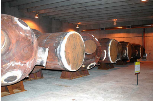
Figure 6.4 Steam generator storage facility. Reproduced with permission from Nuclear Waste Management Division, Ontario Power Generation Inc., 2009. © 2009, Ontario Power Generation Inc.
