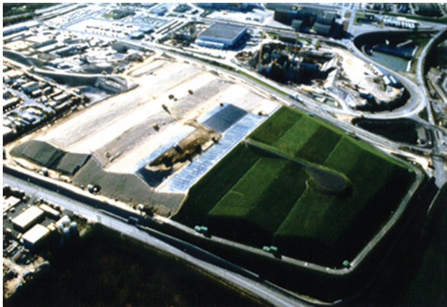
Figure 9.2 (a) Schematic of the La Manche disposal structure. ILW, intermediate-level waste; LLW, low-level waste. Reproduced with permission from J.-M. Potier. © 1998. (b) Photograph of the La Manche disposal facility after closure (Potier and Gallagher, 1998). Reproduced with permission from J.-M. Potier. © 1998
