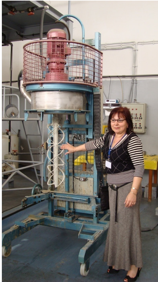
Figure 7.9 Typical cement mixer for centralized waste processing and storage facility. Reproduced with permission from M. Ojovan
