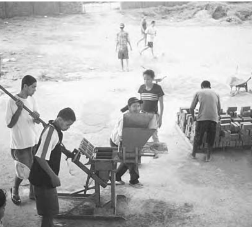
5-12: Students, using a hand-operated press to produce compressed earth blocks. The students formed a cooperative to produce this sustainable resource, with the assistance of Jean D’Aragon and Rosa Fernandez.
