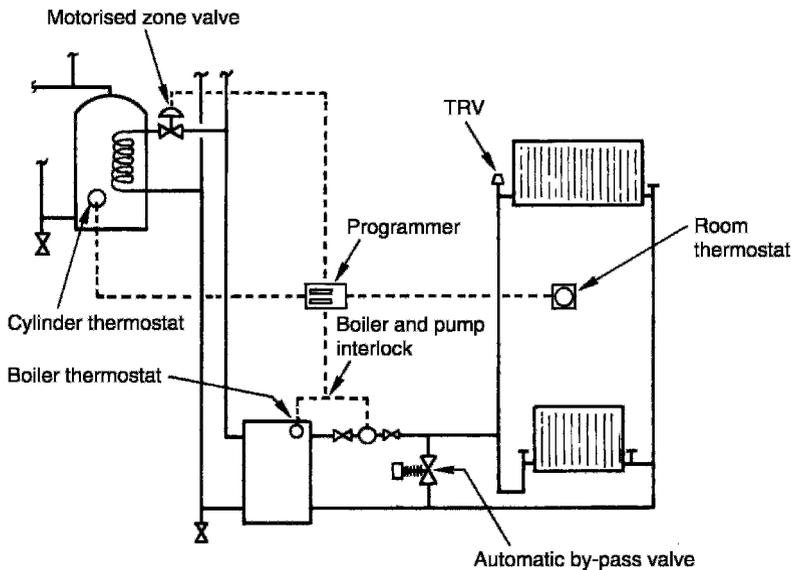
Note: Boiler and pump interlock is the wiring configuration as explained on the previous two pages
