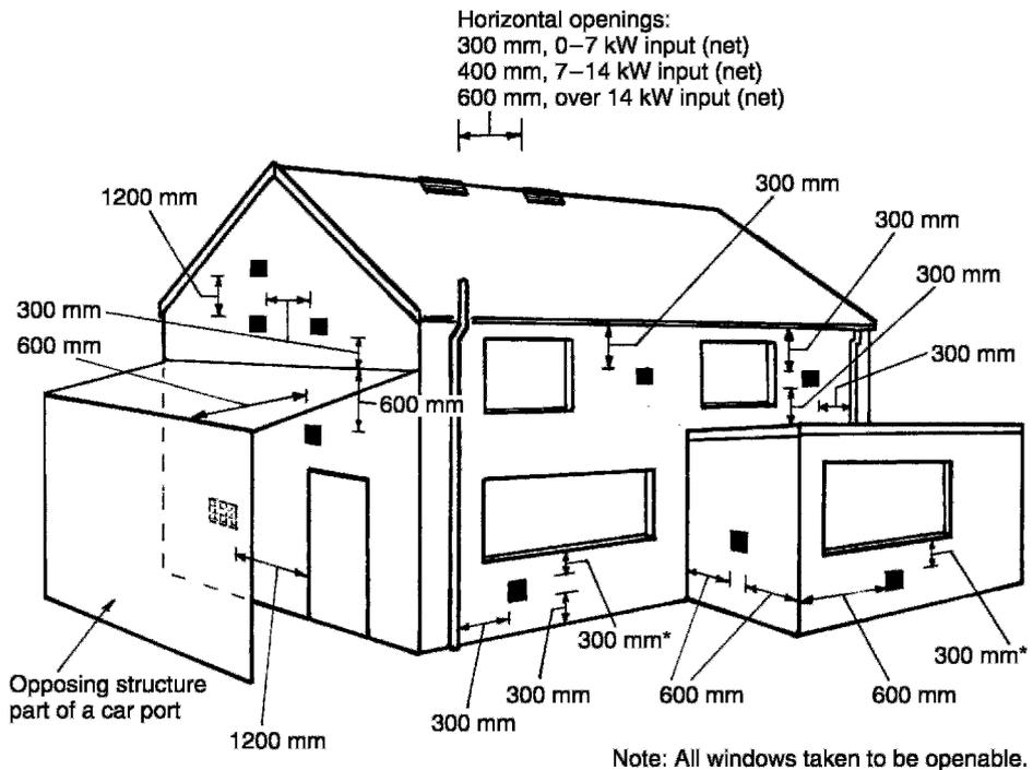
\*0–7 kW input (net) – 300 mm, 7–14 kW input (net) – 600 mm, 14–32 kW input (net) – 1500 mm, over 32 kW input (net) – 2000 mm
