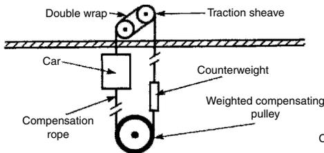
Double wrap 1:1 roped with compensating rope
