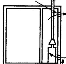
Air vent 1000 mm<sup>2</sup> per kW input (net) for combustion
