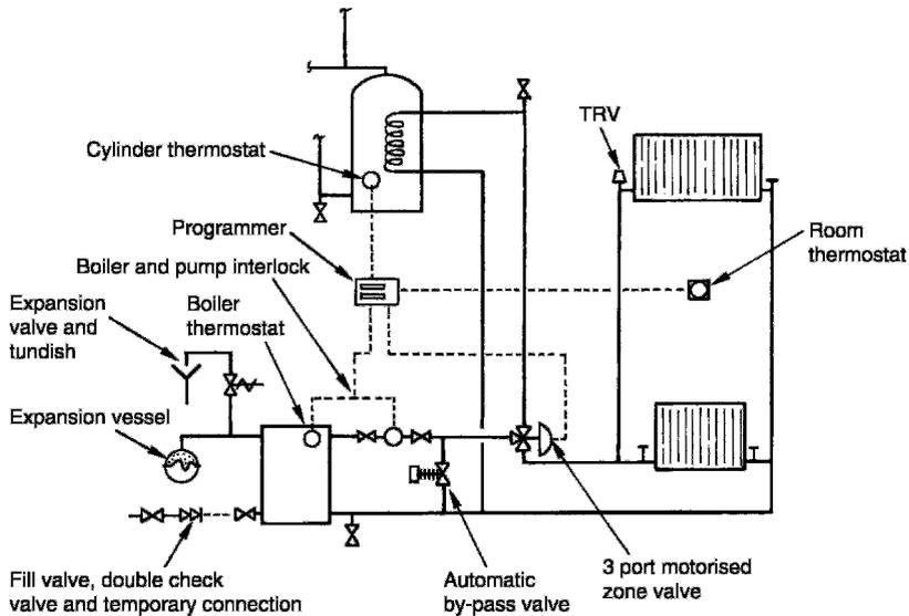
Note: Boiler and pump interlock is the wiring configuration as explained on pages 110 and 111
