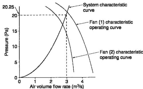
Select fan (1), as with variable settings this would adequately cover the system design characteristics.
