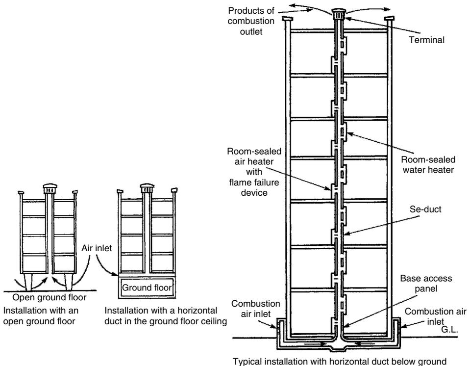
Note: A flame failure device is otherwise known as a flame supervision device.
