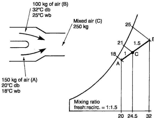
Mixed air (C) = 24.5°C db, 21°C wb, 72% RH and 14 g/kg m.c.
