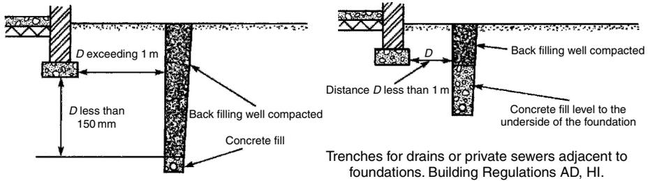
Drains under buildings should be avoided. Where it is impossible to do so, the pipe should be completely protected by concrete and integrated with the floor slab. If the pipe is more than 300 mm below the floor slab, it is provided with a granular surround. Pipes penetrating a wall below ground should be installed with regard for building settlement. Access through a void or with flexible pipe joints each side of the wall are both acceptable.
