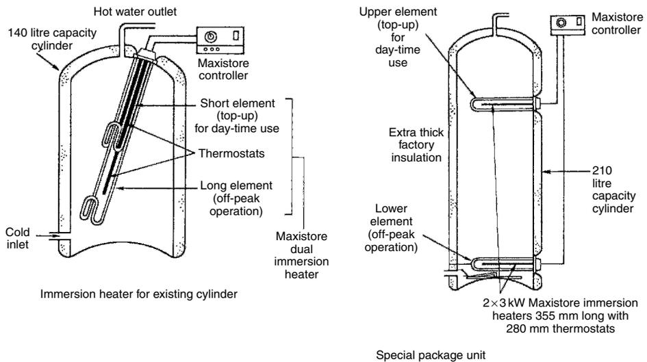
The secondary immersion heater or boost heater is close to the top of the cylinder to ensure that only a limited quantity of water is heated at standard tariff. To maximise economy, the off-peak thermostat is set at 65°C and the boost thermostat at 60°C.
