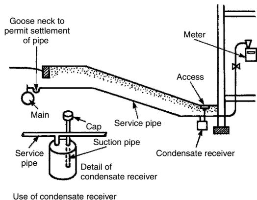
A service pipe is the term given to the pipe between the gas main and the primary meter control. A polyethylene pipe is used underground and steel or copper pipe where it is exposed. Wherever possible, the service pipe should enter the building on the side facing the gas main. This is to simplify excavations and to avoid the pipe having to pass through parts of the substructure which could be subject to settlement. The service pipe must not:
