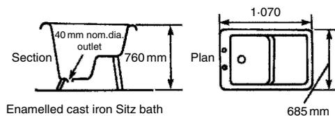
Refs: BS 1189 and 1390: Specifications for baths made from porcelain enamelled cast iron and vitreous enamelled sheet steel, respectively.
