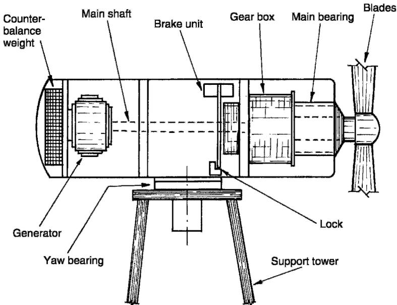
Main components of a wind turbine
