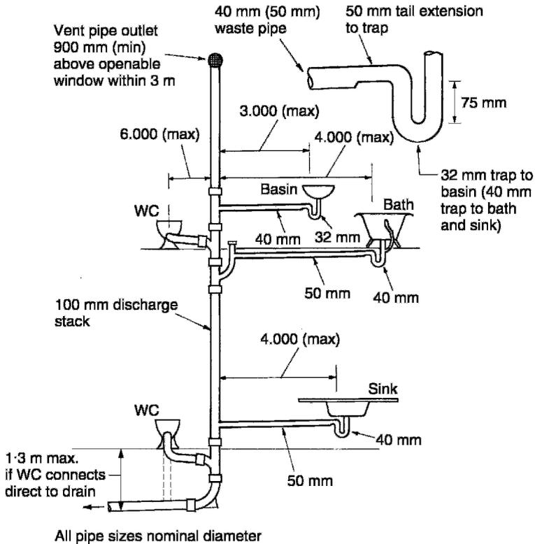
Note: Where larger than standard branch pipes are used, the trap size remains as standard. Each trap is fitted with a 50 mm tail extension before connecting to a larger waste pipe.
