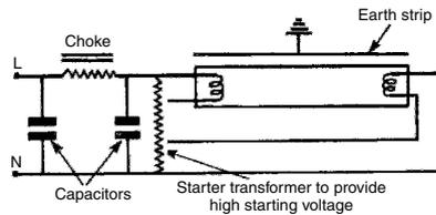
Control gear is needed to start the discharge and to keep the light steady during operation. A transformer provides a quick start.
