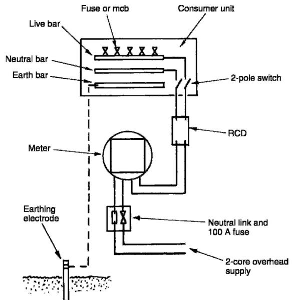
TN-S system - this is widely used in the UK, with the electricity supply company providing an earth terminal with the intake cable. This is usually the metal sheathing around the cable, otherwise known as the supply protective conductor. It connects back to the star point at the area transformer, where it is effectively earthed.
