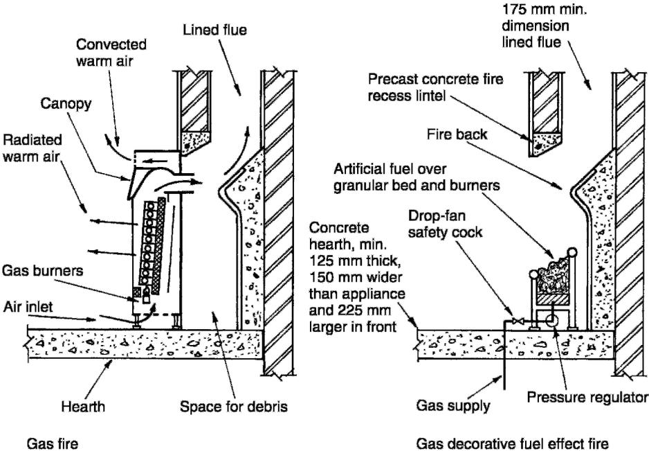
Ref: BS 5871: Specification for installation and maintenance of gas fires, convector heaters, fire/back boilers and decorative fuel effect gas appliances. (In 3 parts).
