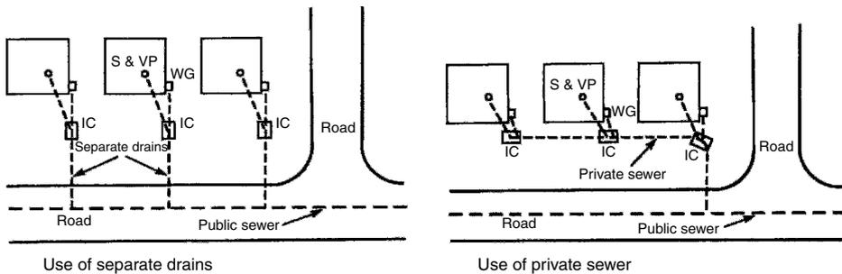
Connection of a drain or private sewer to the public sewer can be made with a manhole. If one of these is used at every connection, the road surface is unnecessarily disrupted. Therefore a saddle is preferred, but manhole access is still required at no more than 90 m intervals. Saddles are bedded in cement mortar in a hole made in the top of the sewer.
