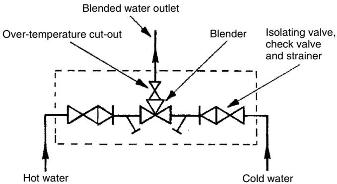
The stored hot water temperature must be at least 60°C to prevent the development of bacteria. Therefore, simply setting the hot water storage cylinder thermostat to provide a general supply of hot water at about 48°C is prohibited. Subject to the local water supply authority's requirements and approval, it may be possible to install just one central or master thermostatic mixing valve, to regulate domestic hot water requirements to all fittings as shown in principle, below.
