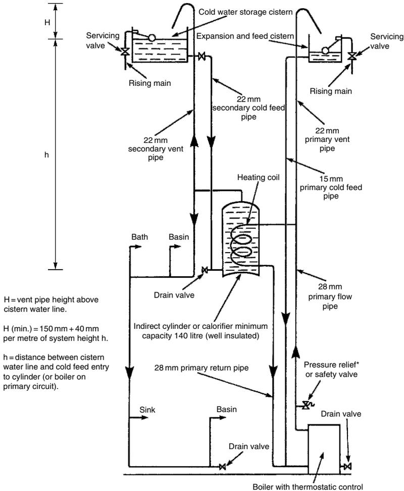
\*A safety valve is not normally required on indirect open vent systems, as in the unlikely occurrence of the primary flow and vent becoming obstructed, water expansion would be accommodated up the cold feed pipe.
