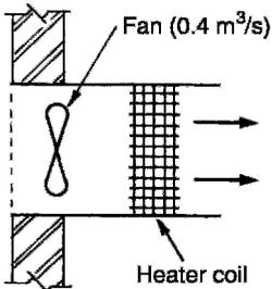
$$\begin{aligned} \text{Heater rating} &= 0.4 \times 1.2 \times 1.0 \times (22 - -4) \\ &= 12.48 \text{ kW} \end{aligned}$$
