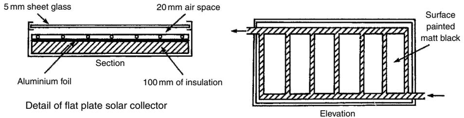
Detail of flat plate solar collector
