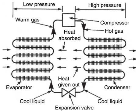
Note:- The flow of the refrigerant can be reversed so that the building is warmed in winter and cooled in summer
