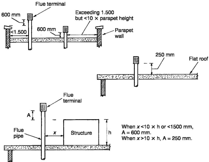
Ref: BS 5440-1: Installation and maintenance of flues and ventilation for gas appliances of rated input not exceeding 70 kW net. Specification.
