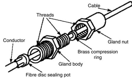
Exploded view of termination joint for mineral insulated copper covered cable
