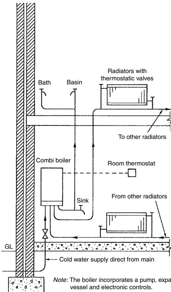
*Note:* The boiler incorporates a pump, expansion vessel and electronic controls. Cold water supply to bath, basin and sink has been omitted for clarity.
