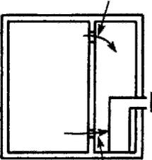
Air vent 1000 mm<sup>2</sup> per kW input (net) for cooling
