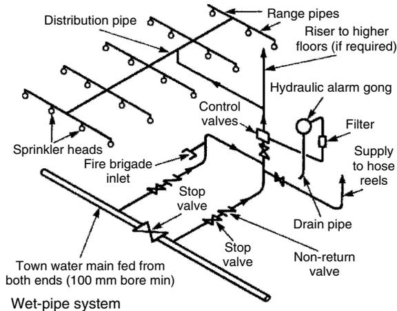
When a sprinkler head is fractured water is immediately dispersed. Water will also flow through an annular groove in the alarm valve seating to a pipe connected to an alarm gong and turbine. A jet of water propels the turbine blades causing the alarm gong to operate. Pipeline flow switches will alert the local fire service in addition to operating an internal alarm system. Except under supervised maintenance, the main stop valve is padlocked in the open position.
