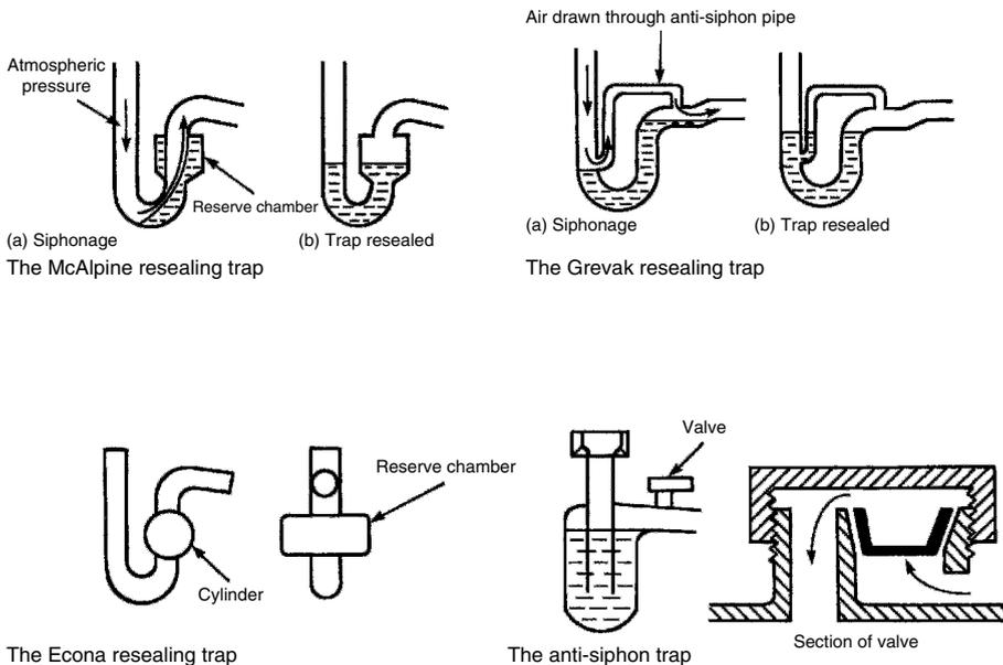
Note: Resealing and anti-siphon traps will require regular maintenance to ensure they are functioning correctly. They can be noisy in use.
