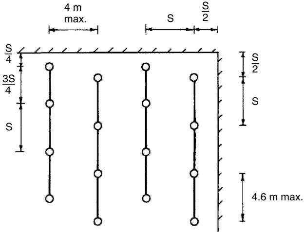
Calculating the number of sprinkler heads: e.g. an ordinary fire hazard category for a factory having a floor area  $20 \text{ m} \times 10 \text{ m}$ .
