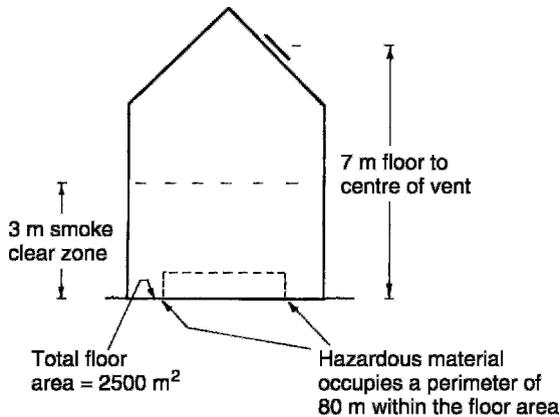
By interpolation, ventilation factor for 7 m approximates to 0.41 m. Ventilator area can be taken as the perimeter occupied by hazardous material, multiplied by the ventilation factor, i.e. 80 m × 0.41 m. This approximates to 33 m<sup>2</sup> or  $(33/2500 \times 100/1) = 1.3\%$  of the floor area.
