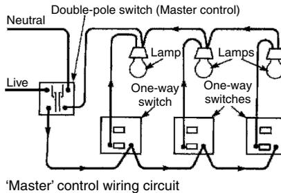
A sub-circuit for lighting is generally limited to a total load of 10, 100 watt light fittings. It requires a 5 amp fuse or 6 amp mcb overload protection at the consumer unit. The importance of not exceeding these ratings can be seen from the simple
