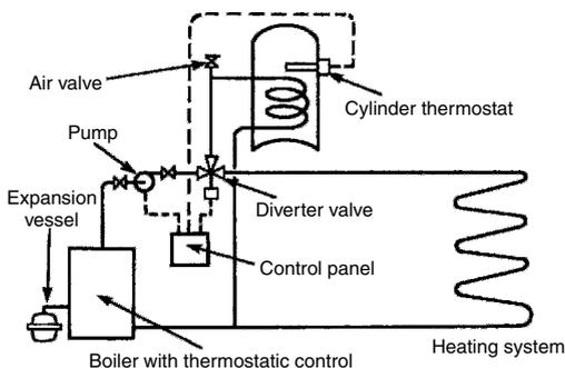
Use of diverter valve to give priority to hot water supply to a system having a pumped circuit to both the heating and the hot water cylinder
