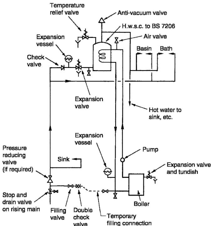
Unvented system with hot water storage capacity in excess of 15 litres, with a sealed primary circuit
