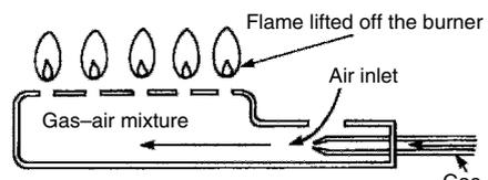
Gas pressure and injector bore correct but with no retention flame
