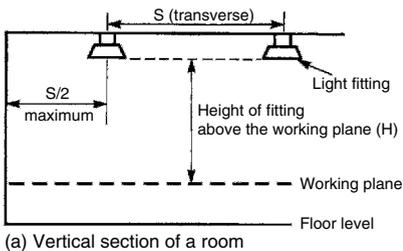
*Example.* An office 8 m long by 7 m wide requires an illumination level of 400 lux on the working plane. It is proposed to use 80 W fluorescent fittings having a rated output of 7375 lumens each. Assuming a utilisation factor of 0.5 and a maintenance factor of 0.8 design the lighting scheme.
