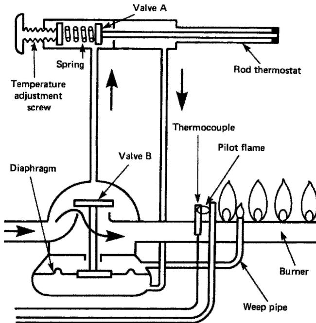
Operating principles of rod thermostat and gas relay valve
