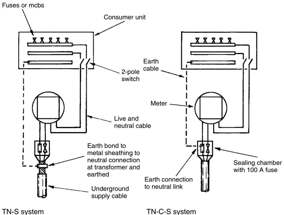
Note: Specification of installation cable between supply company's sealing chamber and consumer's unit - phase/live and neutral 25 mm<sup>2</sup>, earth 10 mm<sup>2</sup> cross-sectional area.
