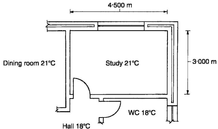
External design temperature  $-1^{\circ}\text{C}$
