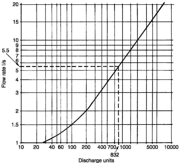
From the chart, a total loading of 832 discharge units can be seen to approximate to 5.5 l/s. A fair comparison with the 5.9 l/s calculated by formula on the preceding page.
