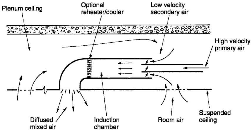
Section through an induction diffuser unit
