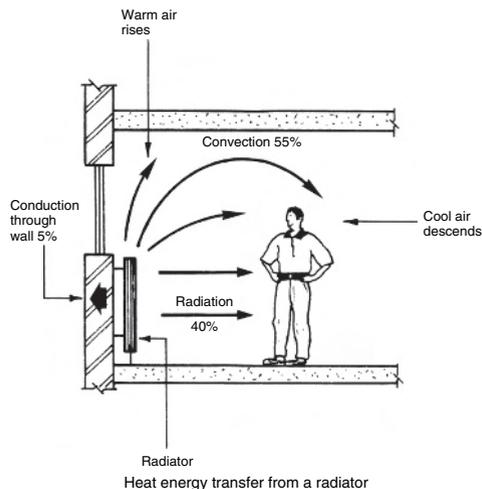
Note: Most heat energy is convected from a radiator, although the term radiator is preferred to differentiate from a convector, where about 90% of heat is convected
