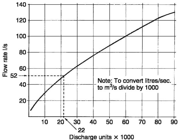
Sewer size can be calculated for a 0.052 m<sup>3</sup>/s flow at half full bore using the formula,  $Q = V \times A$  as shown page 266. Gradient can be calculated using the Chezy and Manning formulas as shown on page 264.
