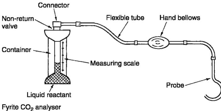
Note: Flue gas samples can be taken by inserting the probe below the draught diverter or through the access plate on top of the appliance combustion chamber. Samples can also be taken at the terminal. The above apparatus is retained to illustrate the principles of probe testing. Modern LCD hand held units are now in general use and have the benefit of determining flue gas temperature, O<sub>2</sub>, CO and CO<sub>2</sub> content.
