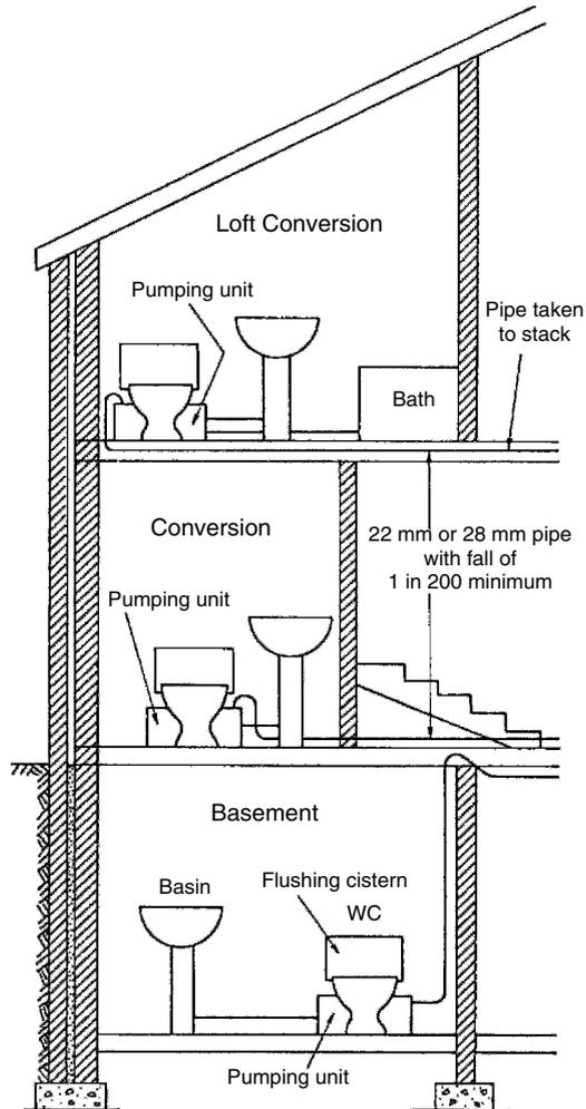
Pipework may be in 22 or 28 mm outside diameter copper tube or equivalent in stainless steel or polypropylene. Easy bends, not elbow fittings must be deployed at changes in direction.
