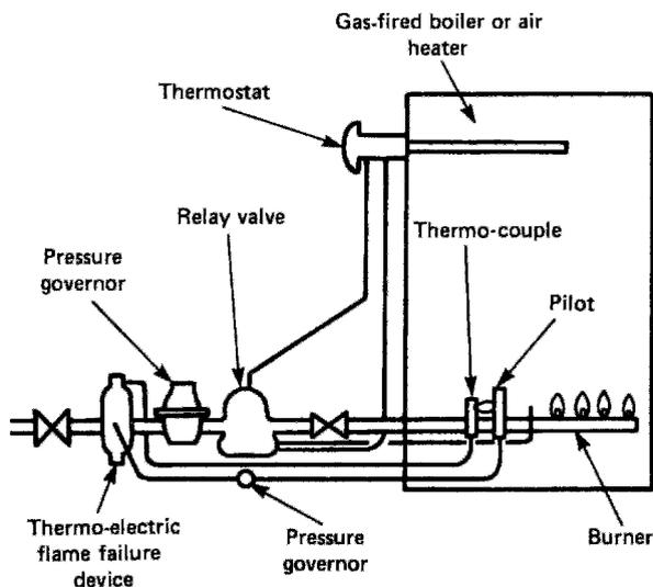
**Gas boiler or air heater controls**
