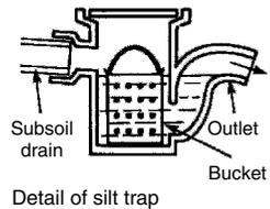
Note: The installation of subsoil drainage may be necessary under the requirements of Building Regulation C3. The purpose of this is to prevent the passage of ground moisture into a building and the possibility of damage to a building.
