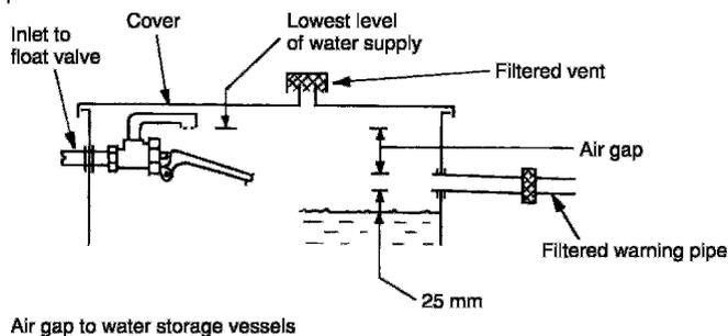
In this situation the air gap should be  $\geq 20$  mm or  $2 \times$  internal diameter of the regulating valve inlet orifice (take greater value).
