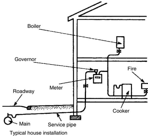
Prior to conversion to natural gas in the 1960s, a condensate receiver was used to trap moisture from town or coal gas where it was impractical to incline the service pipe back to the main.
