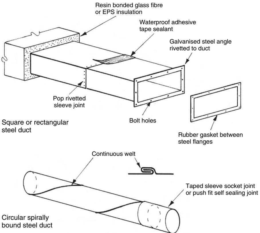
Galvanised sheet steel is the most common material used for ventilation and air conditioning ducting. Factory prefabricated sections are site jointed by bolted steel angle flanges with a rubber sealing gasket, the rigid angles can also function as suspended bracket fixings. Sleeve jointing with pop-rivets and tape sealant is also used with smaller profile sections.
