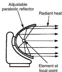
Portable parabolic reflector fire
