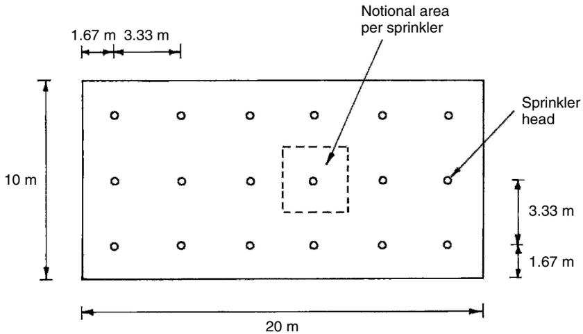
The maximum area served by each sprinkler head =  $3.33 \text{ m} \times 3.33 \text{ m} = 11.1 \text{ m}^2$ .
