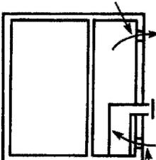
Air vent 500 mm<sup>2</sup> per kW input (net) for cooling
