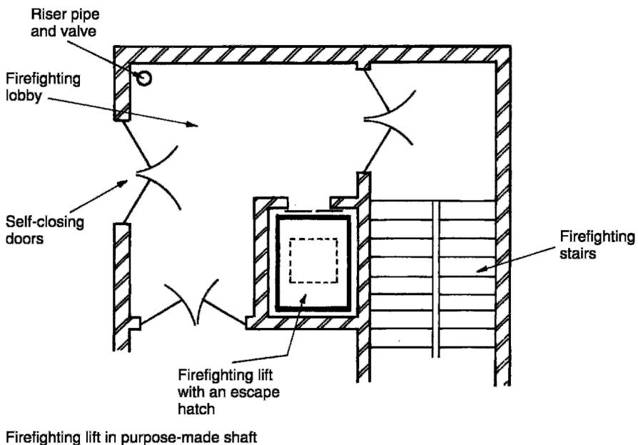
Building Regulations – structures with floors at a height greater than 18 m above fire service vehicle access (usually ground level), or with a basement greater than 10 m below fire service vehicle access, should have accessibility from a purpose-made firefighting lift. All intermediate floors should be served by the lift. Firefighting lifts for other situations are optional as defined in Approved Document B5, Section 18, but will probably be required by the building insurer.
