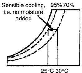
If the air is cooled from 30°C to 25°C the RH = 95%
