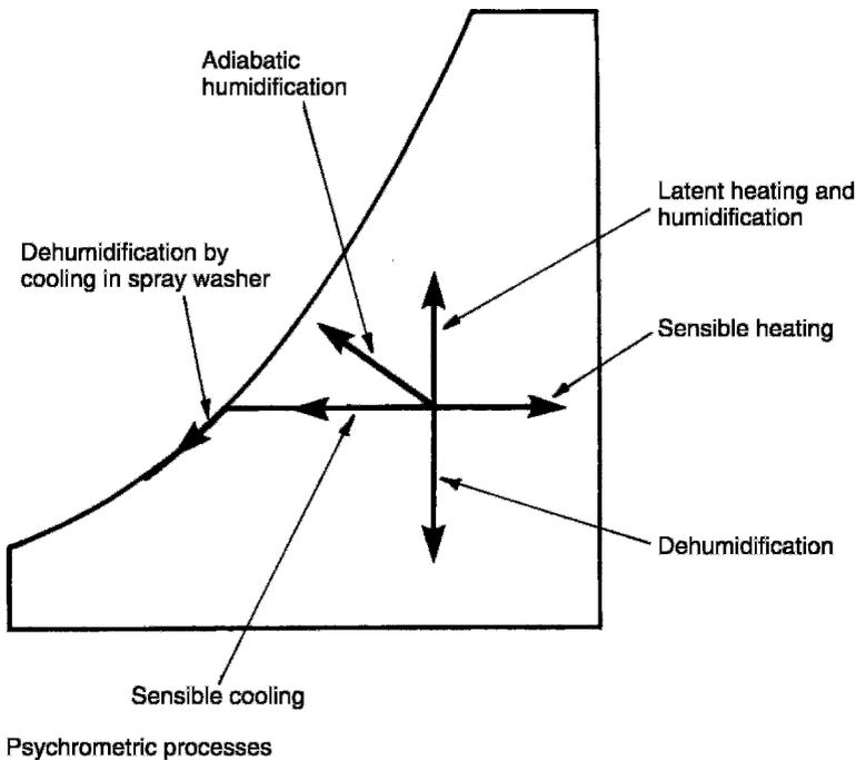
Sensible heating of air may reduce its percentage saturation or relative humidity to an unacceptable level, i.e. <30%. Conversely, sensible cooling may increase the percentage saturation or humidity to an unacceptable level, i.e. >70%.
