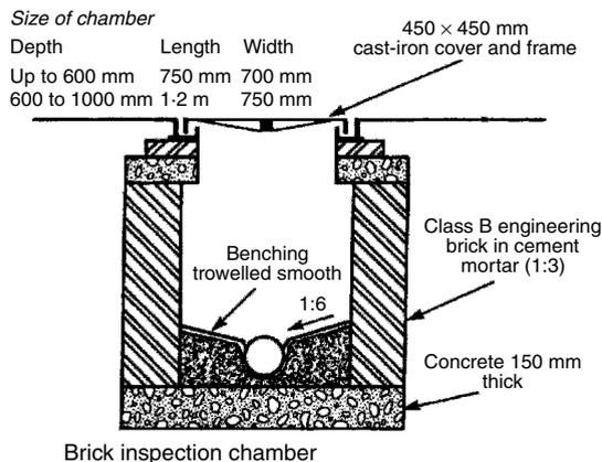
The term manhole is used generally to describe drain and sewer access. By comparison, manholes are large chambers with sufficient space for a person to gain access at drain level. Where the depth to invert exceeds 1 m, step irons should be provided at 300 mm vertical and horizontal spacing. A built-in ladder may be used for very deep chambers. Chambers in excess of 2.7 m may have a reduced area of access known as a shaft (min. 900 × 840 mm or 900 mm diameter), otherwise the following applies:
