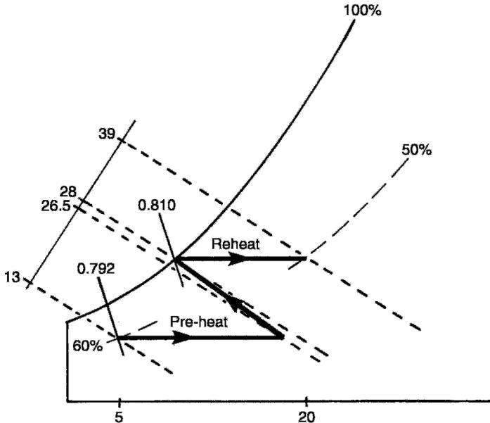
Humidifying by pre-heating, washing and final heating
