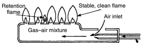
Gas pressure and injector bore correct with a retention flame
