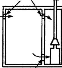
Air vent 2000 mm<sup>2</sup> per kW input (net) for combustion
