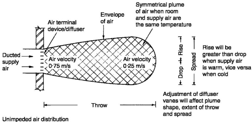
Coanda effect - diffuser location must be selected to avoid unwanted draughts, air delivery impacting on beams, columns and other air deliveries. Where structural elements are adjacent, such as a wall and ceiling, the air delivery may become entrained and drawn to the adjacent surface. This can be advantageous as the plume of air throw, although distorted, may extend to run down the far wall as well.
