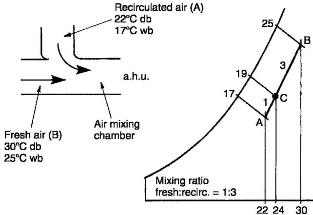
Mixed air condition (C) is found on straight line linking (A) and (B) proportioned 1:3, i.e. 24°C db, 19°C wb, 63% RH and 12g/kg m.c.
