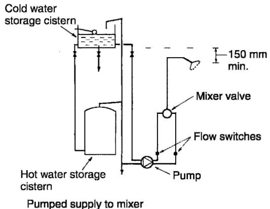
Note: Double check valves may be required on the supply pipes as described on the previous page. The mixing valve and pump may incorporate check valves – refer to manufacturer's information.
