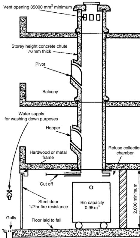
The chute should be circular on plan with a minimum i.d. of 450 mm
