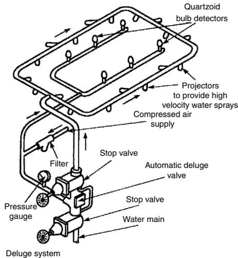
Multiple control system - a heat sensitive sealed valve controls the flow of water to a small group of open sprayers attached to a dry pipe. When a fire occurs, the valve quartzoid bulb shatters allowing the previously retained water to displace the valve stem and flow to the sprayers. An alternative to a heat sensitive valve is a motorised valve activated by a smoke or fire detector.
