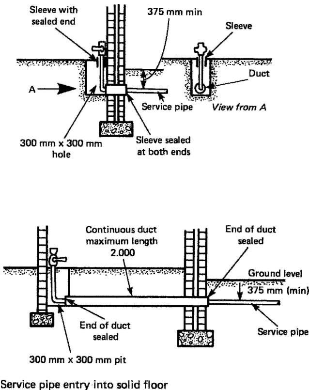
Where a service pipe passes through a wall or a solid concrete floor, it must be enclosed by a sleeve of slightly larger diameter pipe to provide space to accommodate any building settlement or differential movement. The outside of the sleeve should be sealed with cement mortar and the space between the sleeve and service pipe provided with an intumescent (fire resistant) mastic sealant.
