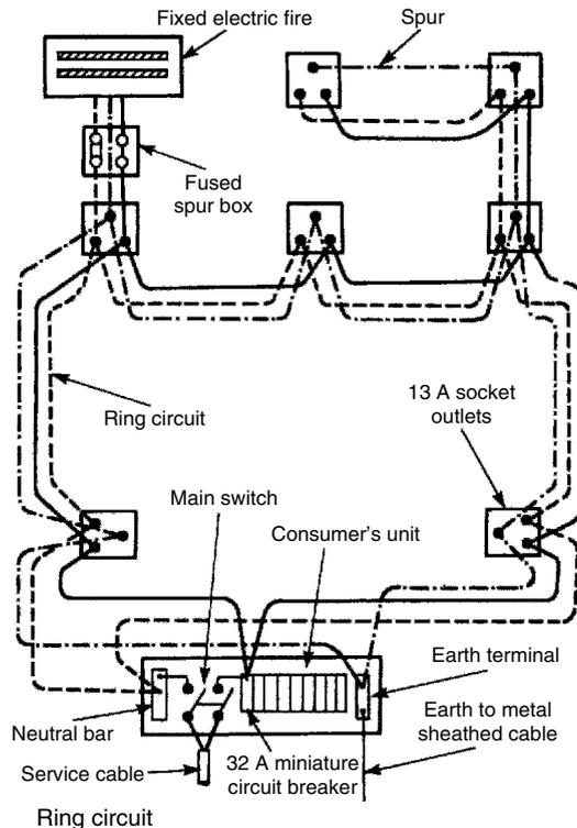
Note: Fixed appliances such as fires, heating controls and low powered water heaters can be connected to a fused spur from a ring socket. Appliances and installations with a load factor above 3 kW, e.g. immersion heater, cooker, extension to an outbuilding, etc. must not be connected to any part of a ring circuit. These are supplied from a separate radial circuit from the consumer unit.
