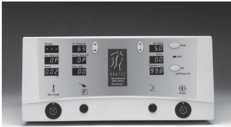
Fig. 14. Intradiscal electrothermal therapy generator. (Courtesy of Smith and Nephew, Menlo Park, CA.)
