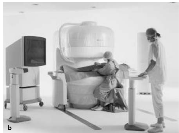
Fig. 19.2. a Open low field MR scanner in “C” configuration (Panorama 0.23T, Philips Medical Systems, Eindhoven, The Netherlands). The image shows the c-arm shaped design. b The image shows an interventional MR imaging scenario. Useful additional equipments are an MR-compatible in-room monitor for navigation and real-time action control as well as an additional workstation panel
