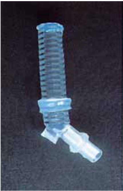
Fig. 10. Cut and unilaterally sealed Dynamic bifurcation stent for the treatment of a stump fistula. Silicone rings around the tracheal and the bronchial limb enhance the sealing effect and help to prevent aspiration.
