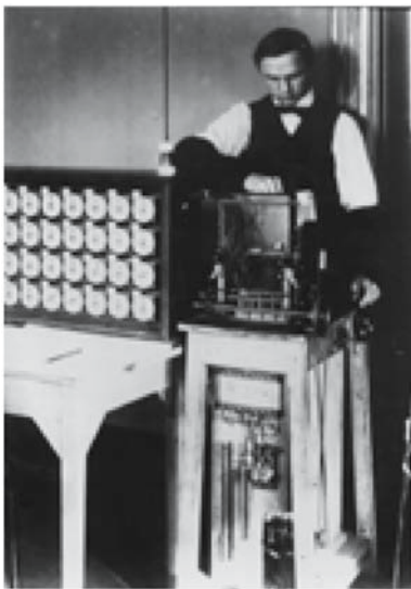
Fig. 1. The Hollerith Tabulating Machine which was developed using punch card technology to speed up the US census counting of Americans in 1880. Photo courtesy of IBM ( http://www-03.ibm.com/ibm/history/history/decade_1890.html )
