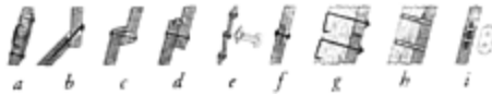
FIG. 1. Constructions of the sides of ships: a , hulk-shaped boats; b , boats of Nachen type (Rhine); c – f , different clinker constructions: c , with short iron nails; d , with rebent iron nails (cogs); e , with iron rivets (Viking ships); f , hidden clinker construction; g – i , carvel constructions: g , with rebent iron nails; h , with treenails; i , mortise-and-tenon construction.
