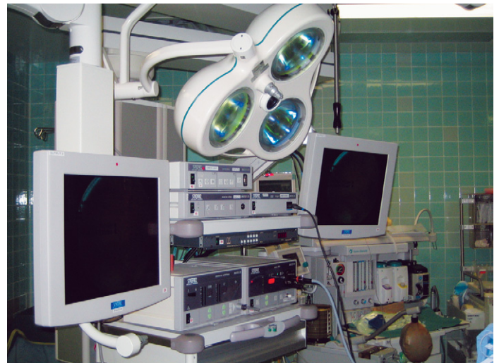
Figure 34-3 Laparoscopic trolley with a camera unit, light source, and insufflator. (Courtesy of Karl Storz Endoscopy, Tuttlingen, Germany.)
