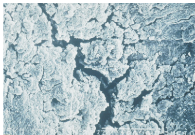
Fig. 7.22 Scanning electron micrograph of a microcrack in bone matrix, showing the fractal pattern of damage.
