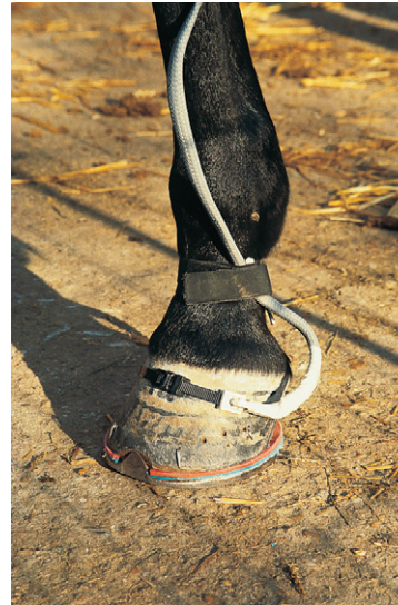
Fig. 12.6 Accelerometer fixed on the hoof to study the shocks and vibrations of the hoof after impact on the ground. The influence of the ground surface and the shoe on the shock damping was studied using this transducer.
