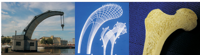
Fig. 7.12 Comparison of the structure and stress distribution of the Fairbairn crane and proximal femur.
