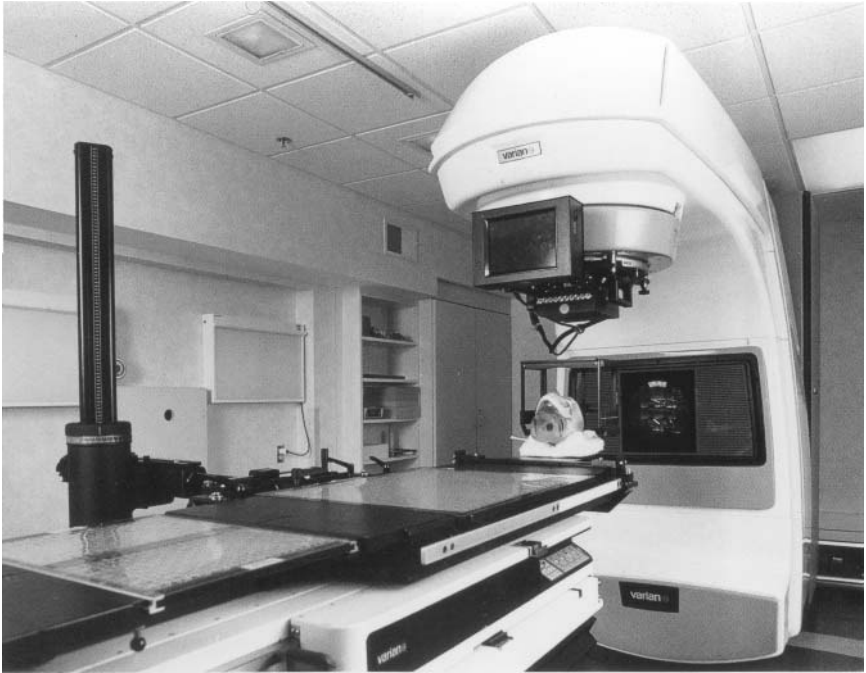
Figure 2.3. A view of the NOMOS MIMiC attached to a Varian accelerator also showing the CRANE. (From NOMOS Corporation brochure.)
