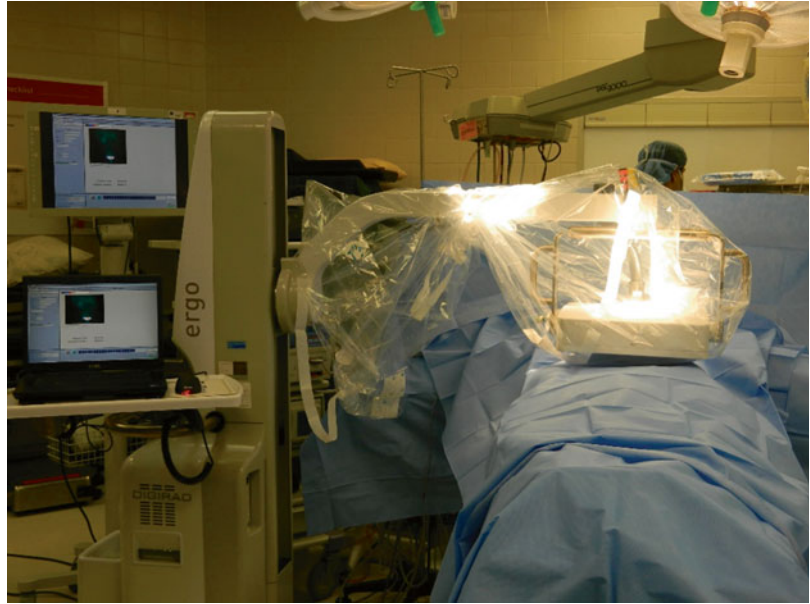
Fig. 3.6 Digital photo demonstrating the intraoperative large field of view PGC (Ergo, Digirad) setup for a pre-incision intraoperative neck image of the parathyroid adenoma (Provided courtesy of Dr. Nathan C. Hall, The Ohio State University Wexner Medical Center, Columbus, USA)
