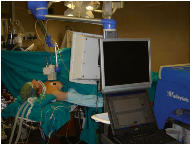
Fig. 23.5 Current device used for ILP. The supporting arm belongs to the new design of portable gamma camera (Sentinella S102). The collimator used is a self-built parallel multi-hole collimator
