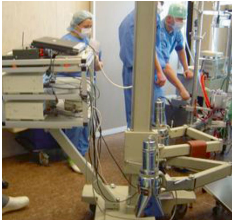
Fig. 23.3 Bulky external detectors used for systemic leakage monitoring during perfusion
