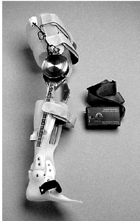
Figure 3. Logical Controlled Electromechanical Free-Knee Long-Leg Orthosis. The control mechanism is attached to the lateral strut of the KAFO at the knee. The electronic control system is in the small box.
