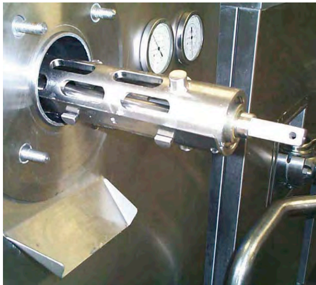
Plate 98 Ice cream Open-type dasher with sharp scraper blades. The dasher is partially inserted into the freezing cylinder of the continuous freezer.
