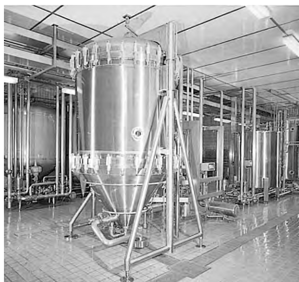
Figure 8 (see color plate 64) Filtration line for 450 hl output per hour; consisting of FILTROstar candle-type precoat filter and PVPP (polyvinyl pyrrolidone, a filter aid dispersed into a cellulose-based matrix) stabilizing plant Filter-o-mat S. Reproduced from Flavour Compounds, Production Methods, Encyclopaedia of Food Science, Food Technology and Nutrition , Macrae R, Robinson RK and Sadler MJ (eds), 1993, Academic Press.
