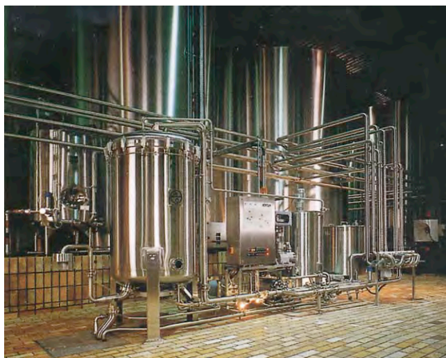
Plate 65 Flavor (Flavour) Compounds Kieselgur filtration plant with 35m 2 filtering area and slurry feeder DOSIMAT 500. Special execution with automatic filtration monitoring. Reproduced from Flavour Compounds, Production Methods, Encyclopaedia of Food Science, Food Technology and Nutrition , Macrae R, Robinson RK and Sadler MJ (eds), 1993, Academic Press.
