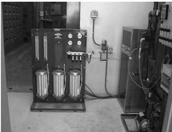
Figure 4 Ozone system installed in a grain-processing plant. Photo courtesy of RGF Environmental Systems.
