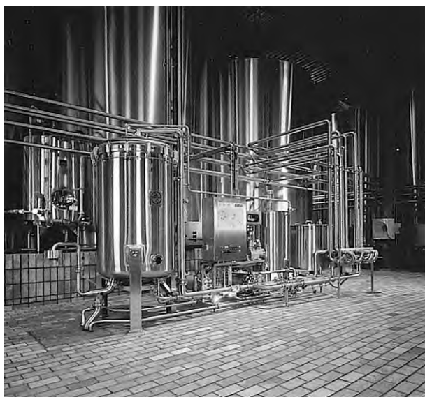
Figure 9 (see color plate 65) Kieselgur filtration plant with 35 m 2 filtering area and slurry feeder DOSIMAT 500. Special execution with automatic filtration monitoring. Reproduced from Flavour Compounds, Production Methods, Encyclopaedia of Food Science, Food Technology and Nutrition , Macrae R, Robinson RK and Sadler MJ (eds), 1993, Academic Press.
