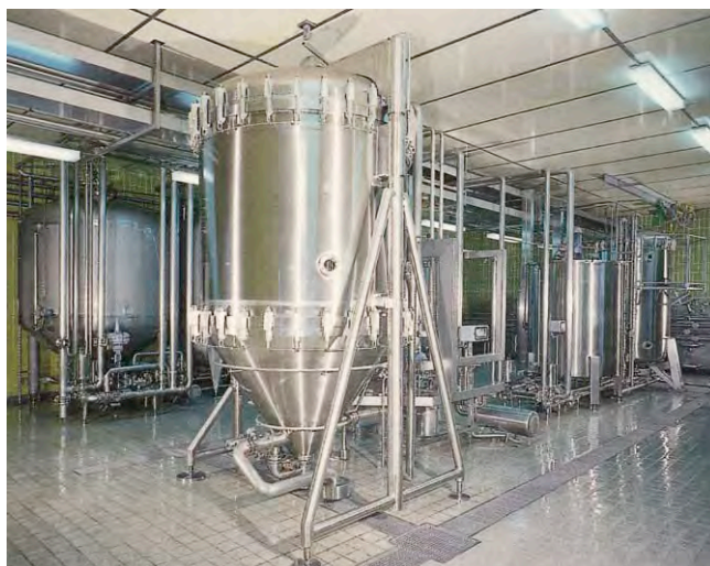
Plate 64 Flavor (Flavour) Compounds Filtration line for 450hl output per hour; consisting of FILTROstar candle-type precoat filter and PVPP (polyvinyl pyrrolidone, a filter aid dispersed into a cellulose-based matrix) stabilizing plant Filter-o-mat S. Reproduce from Flavour Compounds, Production Methods, Encyclopaedia of Food Science, Food Technology and Nutrition , Macrae R, Robinso RK and Sadler MJ (eds), 1993, Academic Press.
