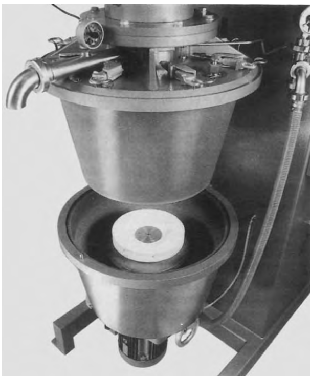
Figure 7 Coball mill. Courtesy of FRYMA-Maschinen AG, Rheinfelden, Switzerland.
