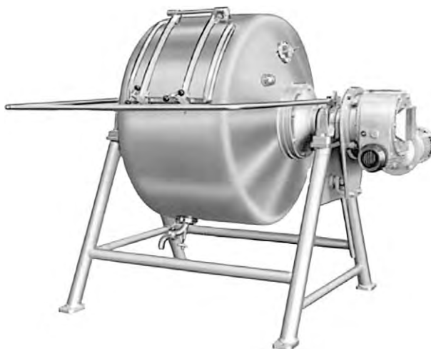
Figure 2 (see color plate 12) Stainless steel batch butter churn (twentieth century). From APV Unit Systems, Denmark, with permission.
