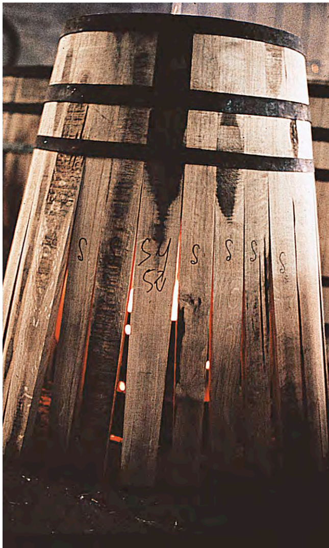
Plate 5 Barrels Preparation for bending with a brazier.
