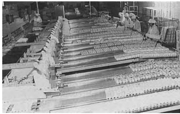
Figure 2 A modern egg-grading and packing machine. Courtesy of Deans Food Group Ltd.
