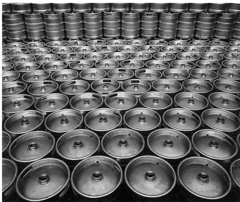
Figure 4 (see color plate 107) Stainless steel's hygienic and corrosion resistance properties are vital in the brewing industry. Today, all new beer barrels are made with type 304 stainless steel. (Courtesy of British Steel plc.)
