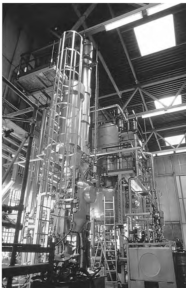
Figure 7 (see color plate 57) Flavor compounds: highly efficient distillation columns. Reproduced from Flavour Compounds, Production Methods, Encyclopaedia of Food Science, Food Technology and Nutrition , Macrae R, Robinson RK and Sadler MJ (eds), 1993, Academic Press.
