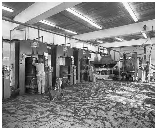
Figure 5 (see color plate 117) Hydraulic pressure unit (courtesy of ELAIS SA, Piraeus, Greece).
