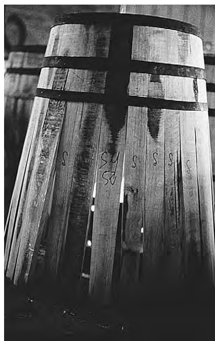
Figure 8 (see color plate 5) Preparation for bending with a brazier.
