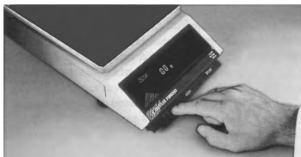
Figure 2 Modern electronic balance with a single control bar. Reproduced from Weighing, Encyclopaedia of Food Science, Food Technology and Nutrition , Macrae R, Robinson RK and Sadler MJ (eds), 1993, Academic Press.
