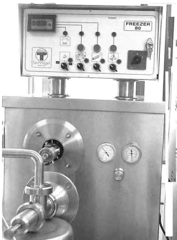
Figure 3 (see color plate 97) Continuous-type freezer with front removed revealing the freezing cylinder and dasher. To regulate the flow of mix and the extent of freezing, pressure is exerted on the freezing chamber by turning the handle located at the outlet for the frozen product in the cylinder cover.
