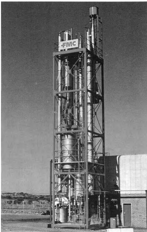
Figure 5 (see color plate 31) Model thermally accelerated short-time evaporator. Courtesy of FMC Food Tech Citrus System, Catania (Sicily) Italy.
