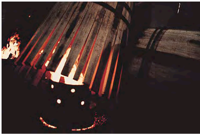
Plate 4 Barrels A barrel placed over a brazier for bending.
