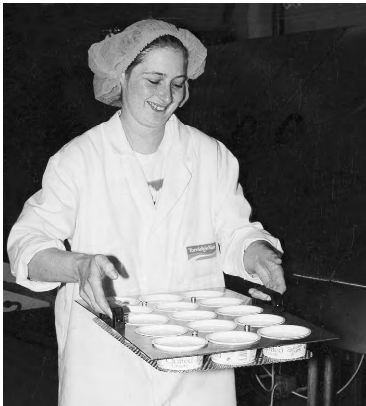
Figure 3 Commercial operator transferring a tray of cream in retail tubs from the scalder to the cooling room.
