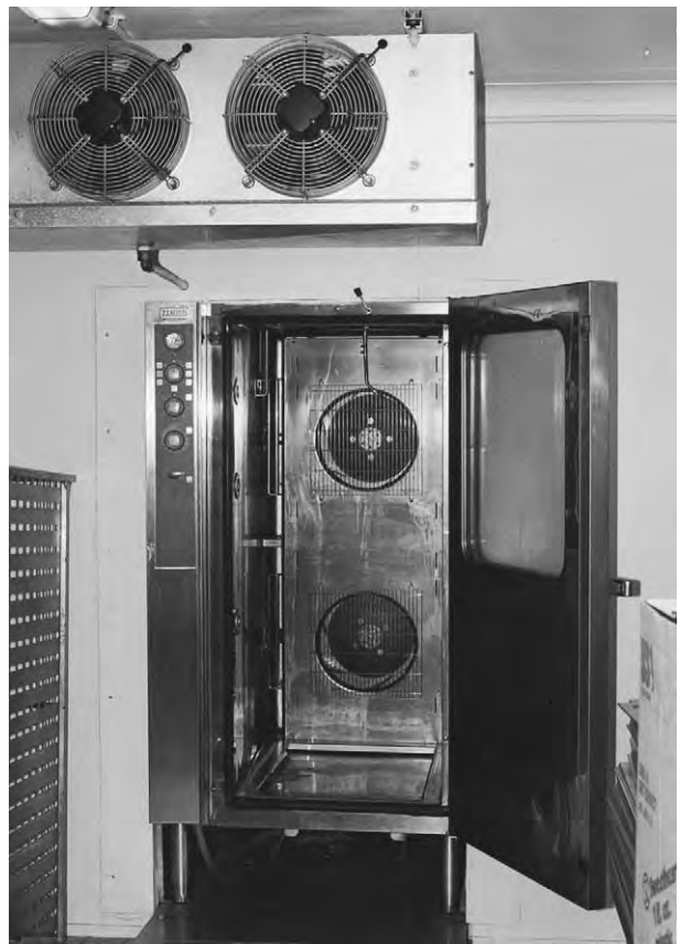
Figure 1 Free-standing hot-air convection oven showing overhead fans and a mobile rack on the left-hand side, which has shelves for retail containers.
