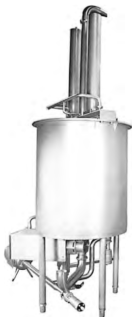
Figure 6 Butter buffer tank. From APV Unit Systems, Denmark, with permission.
