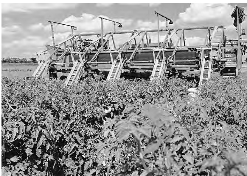
Figure 2 (see color plate 134) Harvest aid for fresh market tomatoes. Fruit are sorted and accumulated on a hopper on the machine. The fruit are periodically transferred to half-tonne bins for transport to the packing house.
