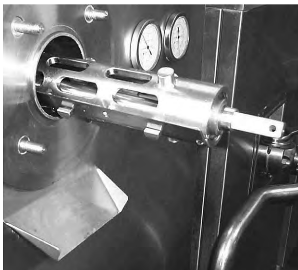
Figure 4 (see color plate 98) Open-type dasher with sharp scraper blades. The dasher is partially inserted into the freezing cylinder of the continuous freezer.
