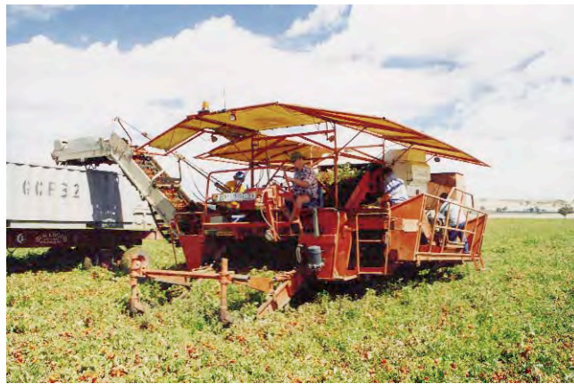
Plate 135 Tomatoes Mechanical harvesting of processing tomatoes. Plants are cut at ground level, and elevated on to a shaker which separates the fruit from the plants.
