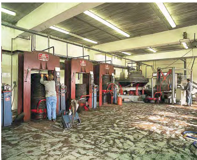
Plate 117 Olive Oil Hydraulic pressure unit (courtesy of ELAIS SA, Piraeus, Greece).
