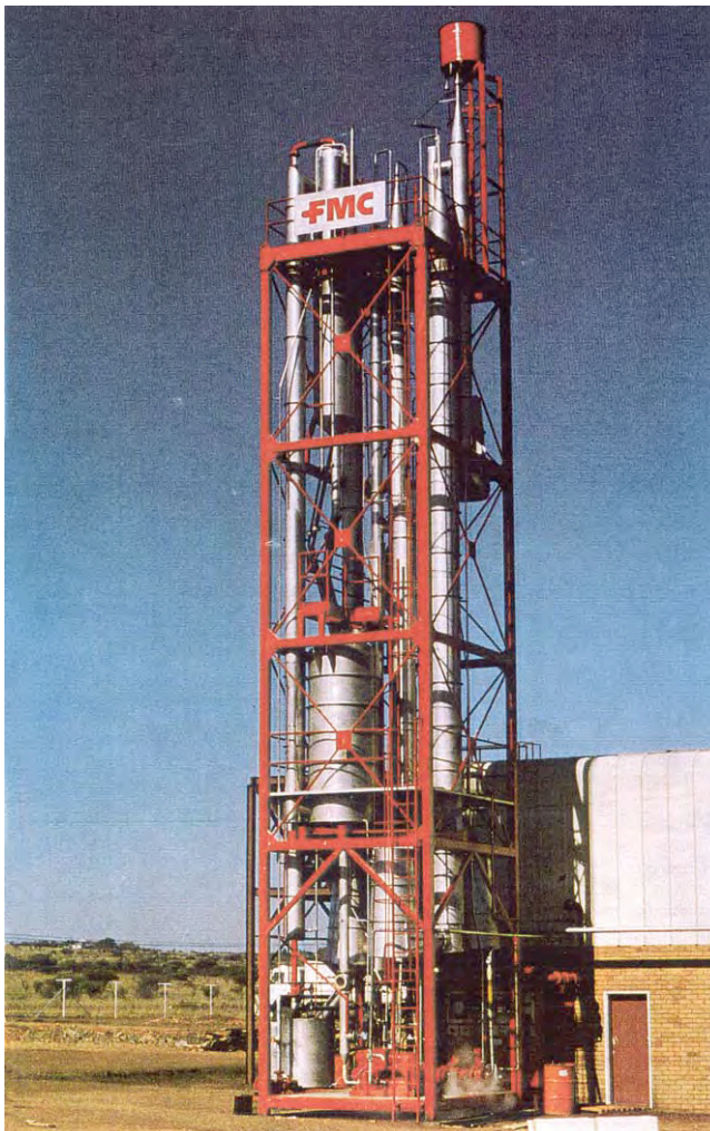
Plate 31 Citrus Fruits Model thermally accelerated short-time evaporator. Courtesy of FMC Food Tech Citrus System, Catania (Sicily) Italy.
