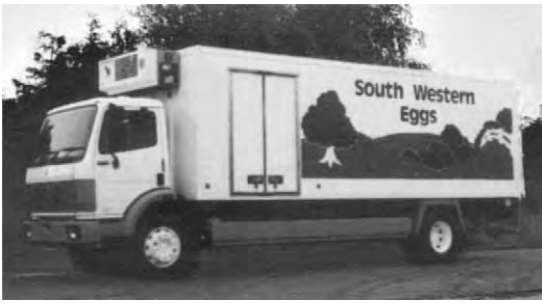
Figure 1 A temperature-controlled egg transporter. Courtesy of Thames Valley Foods Ltd.
