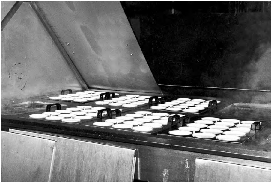
Figure 2 Large bain marie -style scalder, designed with a gabled cover to avoid heat loss.
