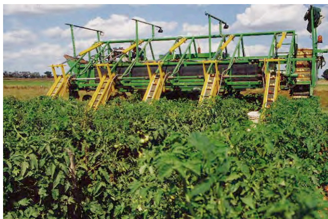
Plate 134 Tomatoes Harvest aid for fresh market tomatoes. Fruit are sorted and accumulated on a hopper on the machine. The fruit are periodically transferred to half-tonne bins for transport to the packing house.
