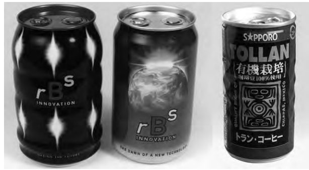
Figure 16 RBS cans and TULC can. From The CanMaker November 1998 and June 1997, Copyright 1998 Sayers Publishing Group Ltd. Reprinted with permission.
