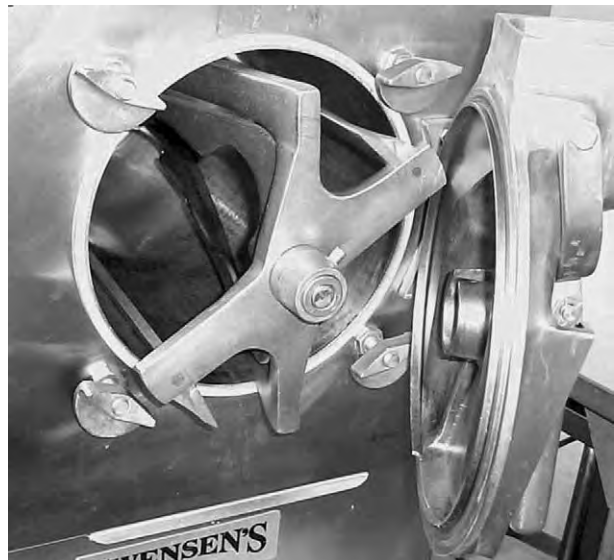
Figure 2 Batch-type ice cream freezer barrel containing beater and blades. The door has an opening through which particulate-type flavorings can be added near the end of the freezing cycle. Frozen product exits through a hatch in the door.
