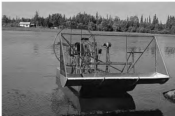
Figure 2 Propeller-driven airboat used to harvest lake-grown wild rice.
