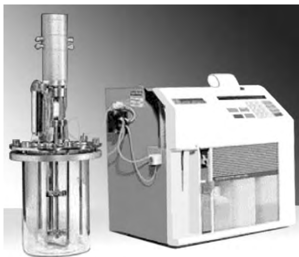
Figure 5 YSI 2700 SELECT™ Biochemical Analyzer. Photo courtesy of YSI incorporated, Yellow Springs, USA.
