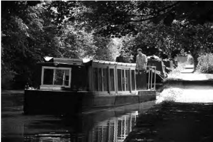
Figure 15.7 The 'Ross Barlow' fuel cell powered narrow boat
