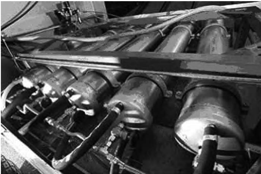
Figure 15.3 Metal hydride storage containers in the Protium Project
