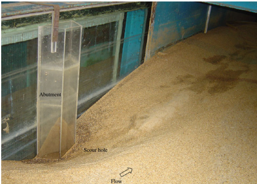
Fig. 10.24 Photograph of an equilibrium scour hole at a wing-wall abutment in a flume
