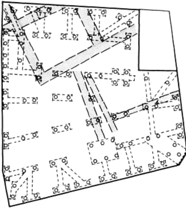
Figure 13.2 Piling arrangements at Micklegate, York before the discovery of Roman remains: the Roman remains are shown by shading. (Source: David Readman.)
