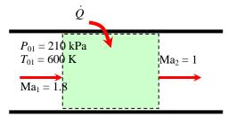
Then the inlet velocity and the mass flow rate become
