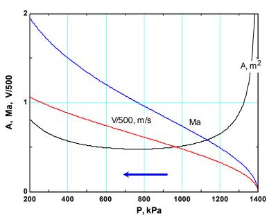
**Discussion** We are assuming that the back pressure is sufficiently low that the flow is choked at the throat, and the flow downstream of the throat is supersonic without any shock waves. Mach number and velocity continue to rise right through the throat into the diverging portion of the nozzle, since the flow becomes supersonic.
