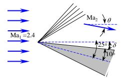
**Solution** Air flowing at a specified supersonic Mach number undergoes a compression turn (an oblique shock) over a tilted wedge. The Mach number, pressure, and temperature downstream of the shock below the wedge are to be determined.
