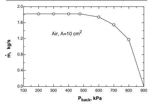
**Discussion** We see from the plot that once the flow is choked at a back pressure of 475.5 kPa, the mass flow rate remains constant regardless of how low the back pressure gets.
