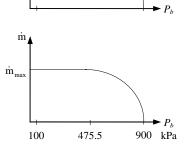
We see from the plots that once the flow is choked at a back pressure of 475.5 kPa, the mass flow rate remains constant regardless of how low the back pressure gets.
