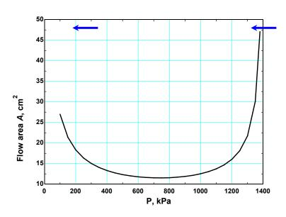
**Discussion** The shape is not actually to scale since the horizontal axis is pressure rather than distance. If the pressure decreases linearly with distance, then the shape *would* be to scale.
