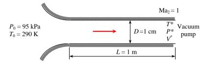
Assumptions 1 The assumptions associated with Fanno flow (i.e., steady, frictional flow of an ideal gas with constant properties through a constant cross-sectional area adiabatic duct) are valid. 2 The friction factor is constant along the duct.
