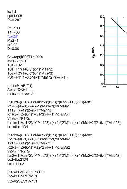
**Discussion** Note that once the flow is choked, any increase in duct length results in a decrease in the mass flow rate and the inlet velocity.
