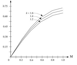
**Discussion** Note that the mass flow rate increases with increasing Mach number and specific heat ratio. It levels off at Ma = 1, and remains constant (choked flow).
