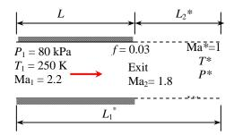
**Assumptions** 1 The assumptions associated with Fanno flow (i.e., steady, frictional flow of an ideal gas with constant properties through a constant cross-sectional area adiabatic duct) are valid. 2 The friction factor remains constant along the duct.
