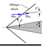
**Solution** Air flowing at a specified supersonic Mach number impinges on a two-dimensional wedge, The shock angle, Mach number, and pressure downstream of the weak and strong oblique shock formed by a wedge are to be determined.
