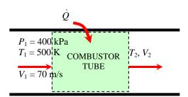
**Solution** Fuel is burned in a rectangular duct with compressed air. For specified heat transfer, the exit temperature and Mach number are to be determined.
