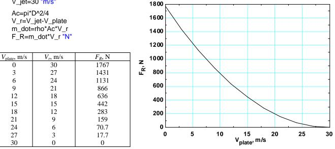
*Discussion* When the plate velocity reaches 30 m/s, there is no relative motion between the jet and the plate; hence, there can be no force acting.
