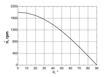
**Discussion** The maximum rpm occurs when  $\theta = 0^{\circ}$ , as expected, since this represents purely tangential outflow. When  $\theta = 90^{\circ}$ , the rpm drops to zero, as also expected, since the outflow is purely radial and therefore there is no torque to spin the sprinkler.
