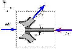
**Solution** A two-armed sprinkler is used to water a garden. For specified flow rate and discharge angles, the rates of rotation of the sprinkler head are to be determined.
