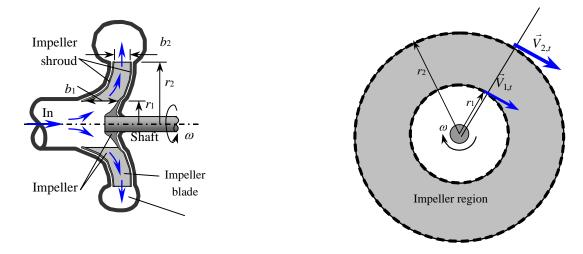
Assumptions 1 The flow is steady in the mean. 2 Irreversible losses are negligible. 3 The tangential components of air velocity at the inlet and the outlet are said to be equal to the impeller velocity at respective locations.
