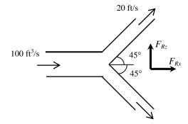
We take the splitting section of water jet, including the splitter as the control volume, and designate the entrance by 1 and the outlet of either arm by 2 (both arms have the same velocity and mass flow rate). We also designate the horizontal coordinate by x with the direction of flow as being the positive direction and the vertical coordinate by z.
