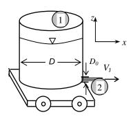
The momentum equation for steady one-dimensional flow is  $\sum \vec{F} = \sum_{\text{out}} \beta \dot{m} \vec{V} - \sum_{\text{in}} \beta \dot{m} \vec{V}$ . Applying it to the water tank,
