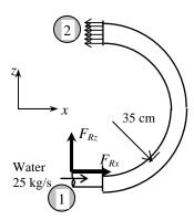
and  $F_R = F_{Rx} = -218$  N since the *y*-component of the anchoring force is zero. Therefore, the anchoring force has a magnitude of 218 N and it acts in the negative *x* direction.
