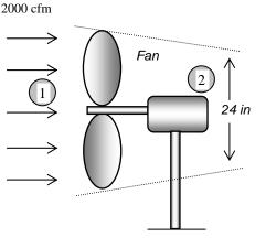
The momentum equation for steady one-dimensional flow is  $\sum \vec{F} = \sum_{\text{out}} \beta \dot{m} \vec{V} - \sum_{\text{in}} \beta \dot{m} \vec{V}$ . Letting the reaction force to hold
