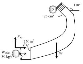
Taking the center of the inlet cross section as the reference level ( $z_1 = 0$ ) and noting that  $P_2 = P_{atm}$ , the Bernoulli equation for a streamline going through the center of the reducing elbow is expressed as
