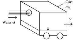
We take the cart as the moving control volume. The net force acting on the cart in this case is equal to the momentum flux of the water jet. Newton's  $2^{nd} \log F = ma = d(mV)/dt$  in this case can be expressed as
