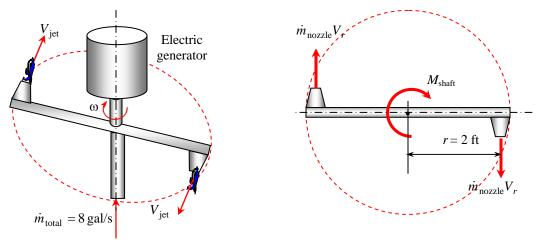
Assumptions 1 The flow is uniform and steady. 2 The water is discharged to the atmosphere, and thus the gage pressure at the nozzle outlet is zero. 3 The nozzle diameter is small compared to the moment arm, and thus we use average values of radius and velocity at the outlet.
