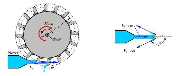
Assumptions 1 The flow is uniform and cyclically steady. 2 The water is discharged to the atmosphere, and thus the gage pressure at the nozzle outlet is zero. 3 Friction and losses due to air drag of rotating components are neglected. 4 The nozzle diameter is small compared to the moment arm, and thus we use average values of radius and velocity at the outlet.
