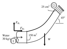
Taking the center of the inlet cross section as the reference level ( $z_1 = 0$ ) and noting that  $P_2 = P_{\text{atm}}$ , the Bernoulli equation for a streamline going through the center of the reducing elbow is expressed as
