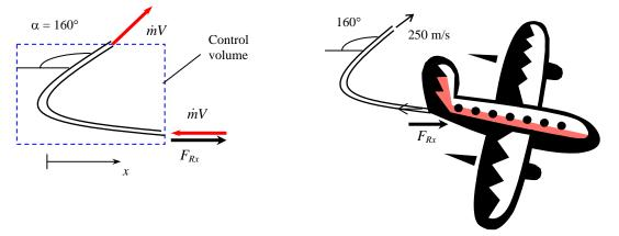
**Discussion** This problem can be solved more generally by measuring the reversing angle from the direction of exhaust gases ( $\alpha = 0$  when there is no reversing). When  $\alpha < 90^{\circ}$ , the reversed gases are discharged in the negative *x* direction, and the momentum equation reduces to
