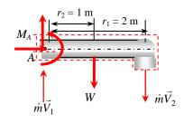
(a) **Downward discharge**: To determine the moment acting on the pipe at point A, we need to take the moment of all forces and momentum flows about that point. This is a steady and uniform flow problem, and all forces and momentum flows are in the same plane. Therefore, the angular momentum equation in this case can be expressed as  $\sum M = \sum_{\text{out}} r\dot{m}V - \sum_{\text{in}} r\dot{m}V$  where r is the moment arm, all moments in the counterclockwise direction are positive, and all
