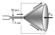
The negative value for  $F_{Rx}$  indicates that the assumed direction is wrong, and should be reversed. Therefore, a force of 518 N must be applied to the cone in the opposite direction to flow to hold it in place. No holding force is necessary in the vertical direction due to symmetry and neglecting gravitational effects.
