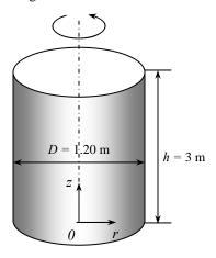
Assumptions 1 The increase in the rotational speed is very slow so that the liquid in the container always acts as a rigid body. 2 Gasoline is an incompressible substance.
