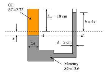
Discussion Note that the fluid levels in the two arms of a U-tube can be different when two different fluids are involved.
