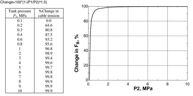
*Discussion* The change in cable tension is at first very rapid, but levels off as the balloon shrinks to nearly zero diameter at high pressure.
