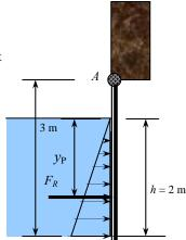
Compared to the previous problem (with higher water depth), the force is much smaller, as expected. Also, Discussion the center of pressure on the gate is much lower (closer to the ground) for the case with the lower water depth.
