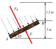
The distance of the pressure center from the free surface of water along the plane of the gate is
