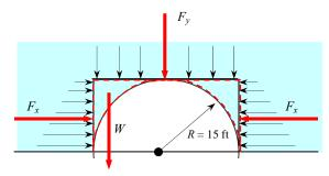
**Solution** A hemispherical dome on a level surface filled with water is to be lifted by attaching a long tube to the top and filling it with water. The required height of water in the tube to lift the dome is to be determined.
