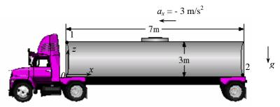
*Assumptions* 1 The acceleration remains constant. 2 Milk is an incompressible substance.
