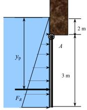
Discussion You can calculate the force at point B required to hold back the gate by setting the net moment around hinge point A to zero.
