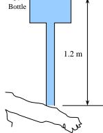
*Discussion* Note that the height of the reservoir can be used to control flow rates in gravity driven flows. When there is flow, the pressure drop in the tube due to friction should also be considered. This will result in raising the bottle a little higher to overcome pressure drop.
