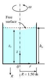
Assumptions 1 The increase in the rotational speed is very slow so that the liquid in the container always acts as a rigid body. 2 Milk is an incompressible substance.
